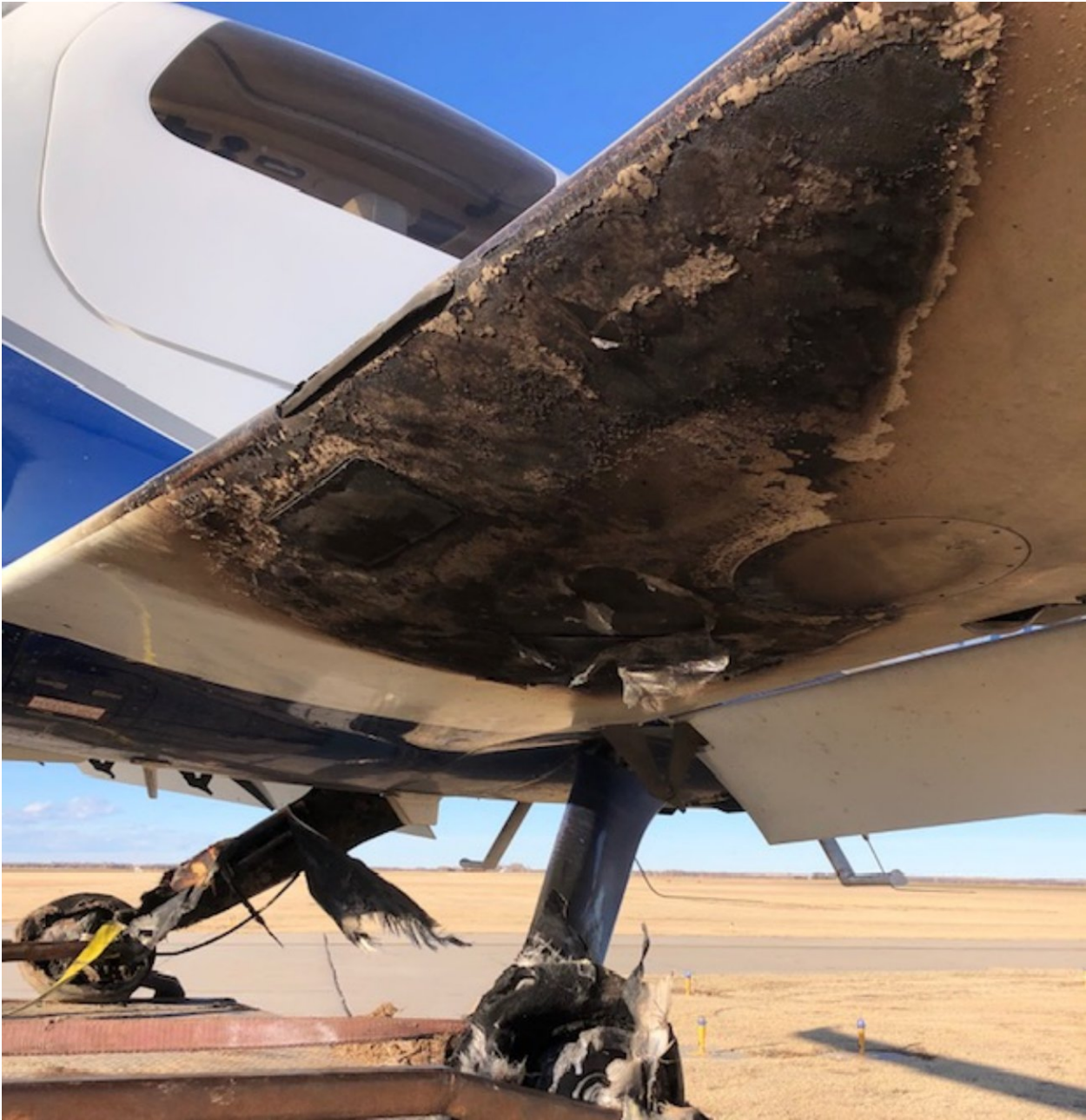
Figure. Fire damage to the main wheel assemblies and underside of the left wing (Source: Federal Aviation Administration).
