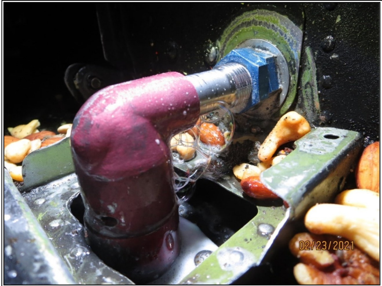
Figure 1: view of fuel line leak (photo provided by MD Helicopters)
