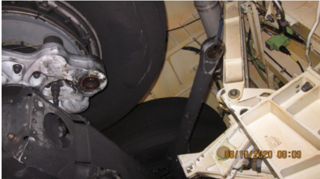
Figure 3. Location of brake rod during postaccident examination (Source: FedEx).
