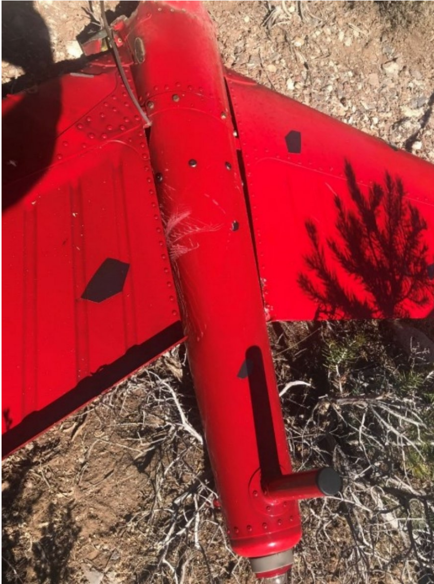
Figure 2. Tail cone and vertical fin displaying cable abrasions
