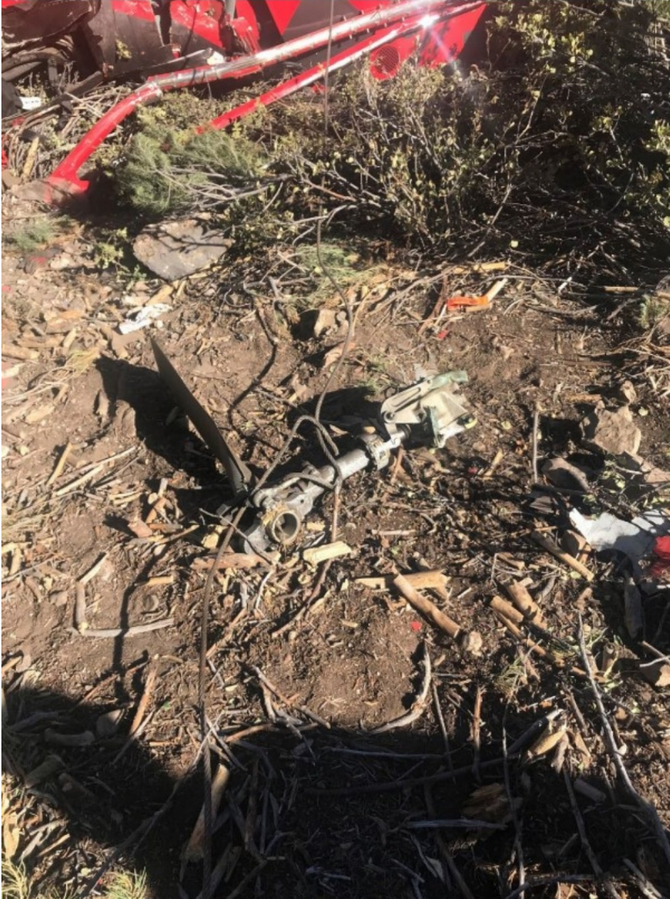
Figure 1. Photo of tail rotor wrapped with cable
