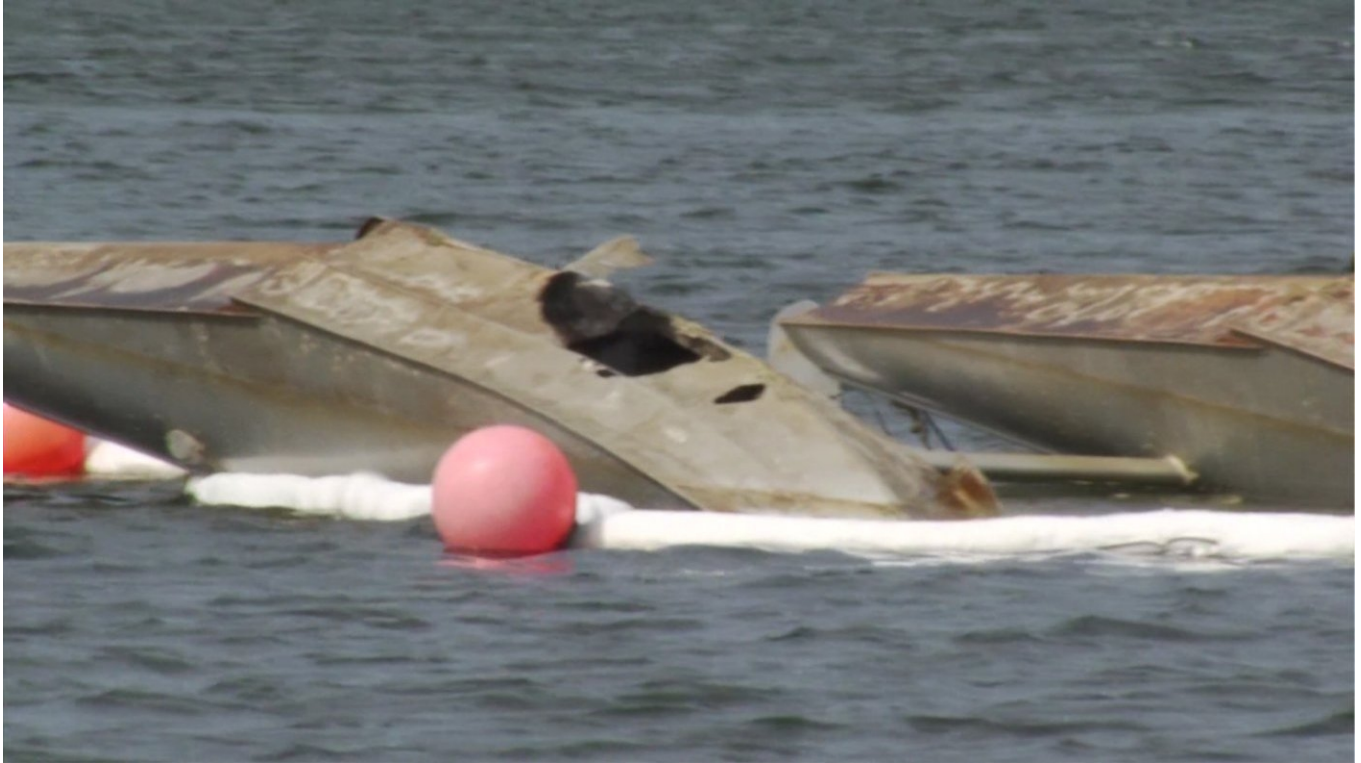
Figure 1 - Accident airplane at accident site, hole visible in left float. Photo courtesy of KTVA.
