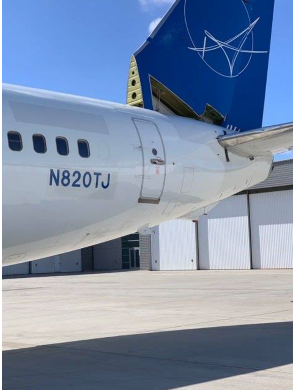
Figure 1. Location of missing dorsal fin and vertical stabilizer panels (Source: FAA).
