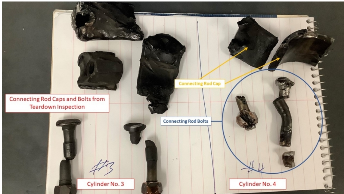
Figure 2: Cylinder No. 3 and 4 Connecting Rod Caps and Bolts Retained from Teardown Inspection
