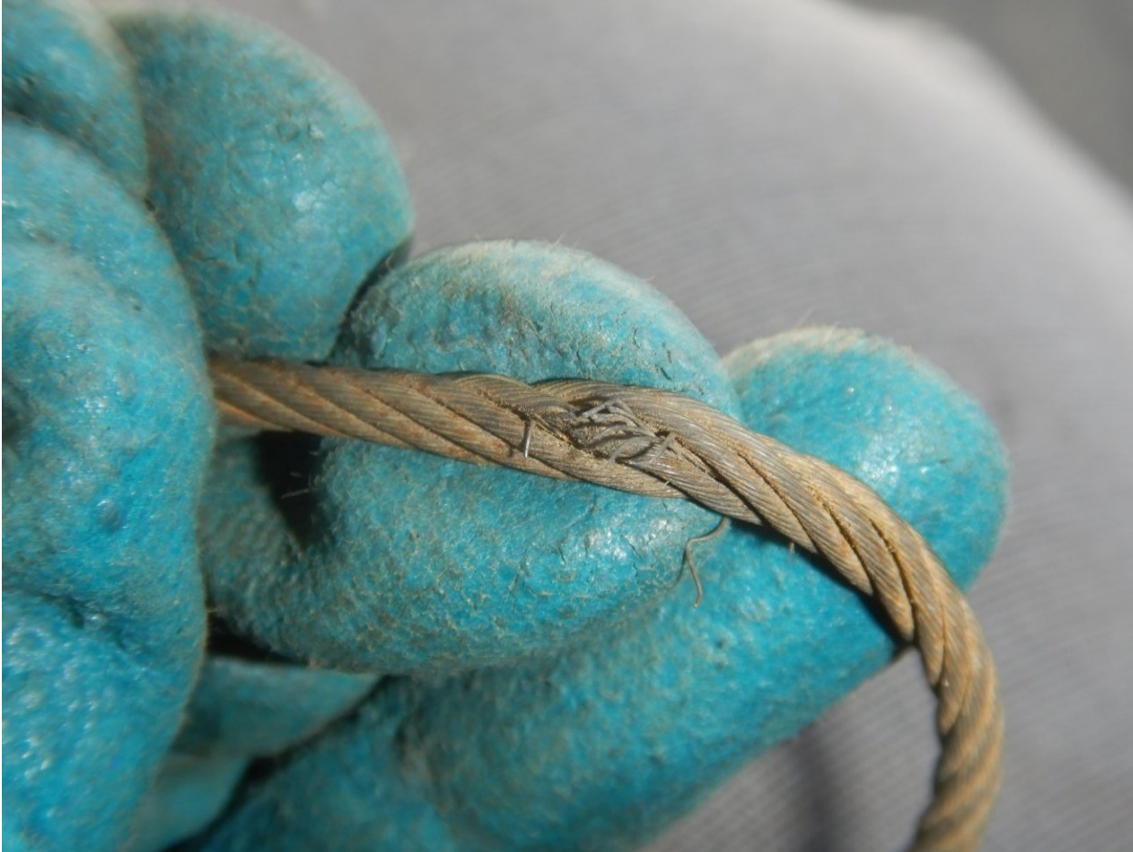
Figure 3. The aileron control cable, showing frayed wires.
