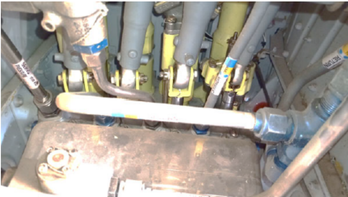
Figure 3. Red arrow denotes small pool of hydraulic fluid visible to the right of the auxiliary servo cylinder. (Image courtesy of CHI Aviation)
