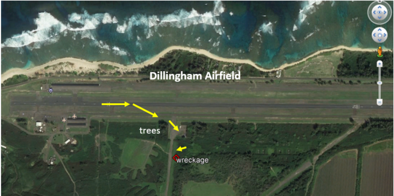
Figure 1. Google Earth image of runway 8 and estimated flightpath (yellow) based on witness statements.
