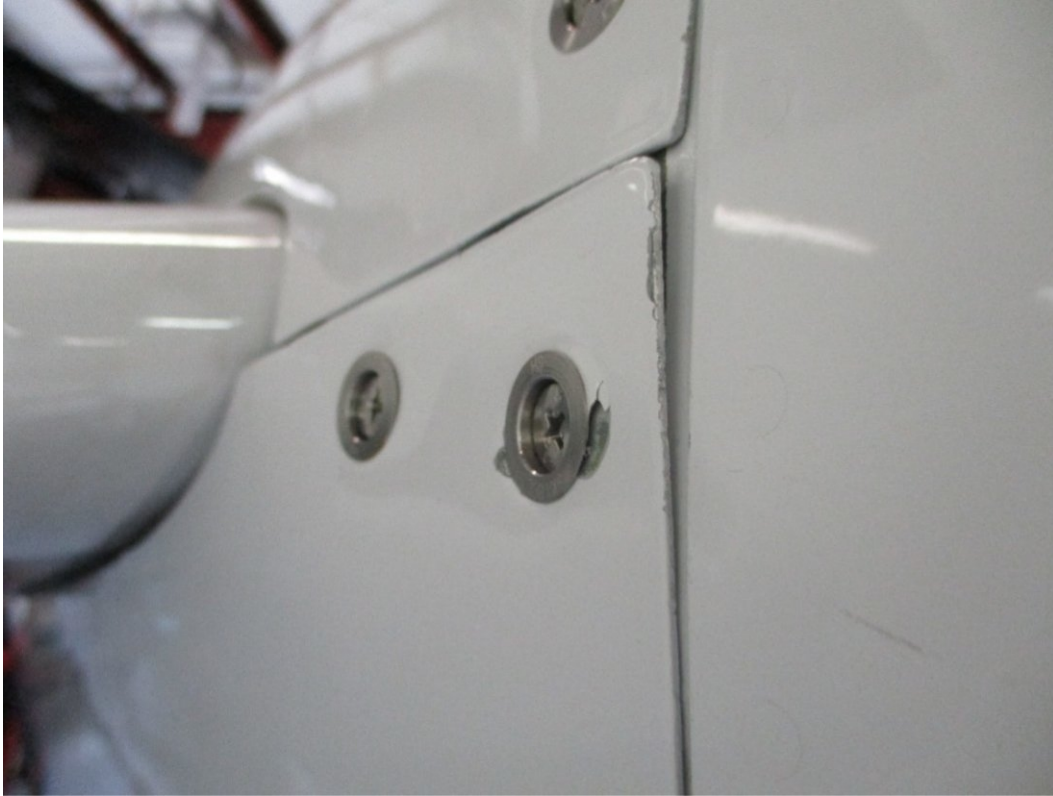
Figure 4: Shows the left engine inboard lower cowl mismatch and screw heads recessed beneath their grommets at the same relative receptacle location numbers 10 and 11. The grommets were labeled “HS SKYBOLT” and the studs were labeled “-3.”
