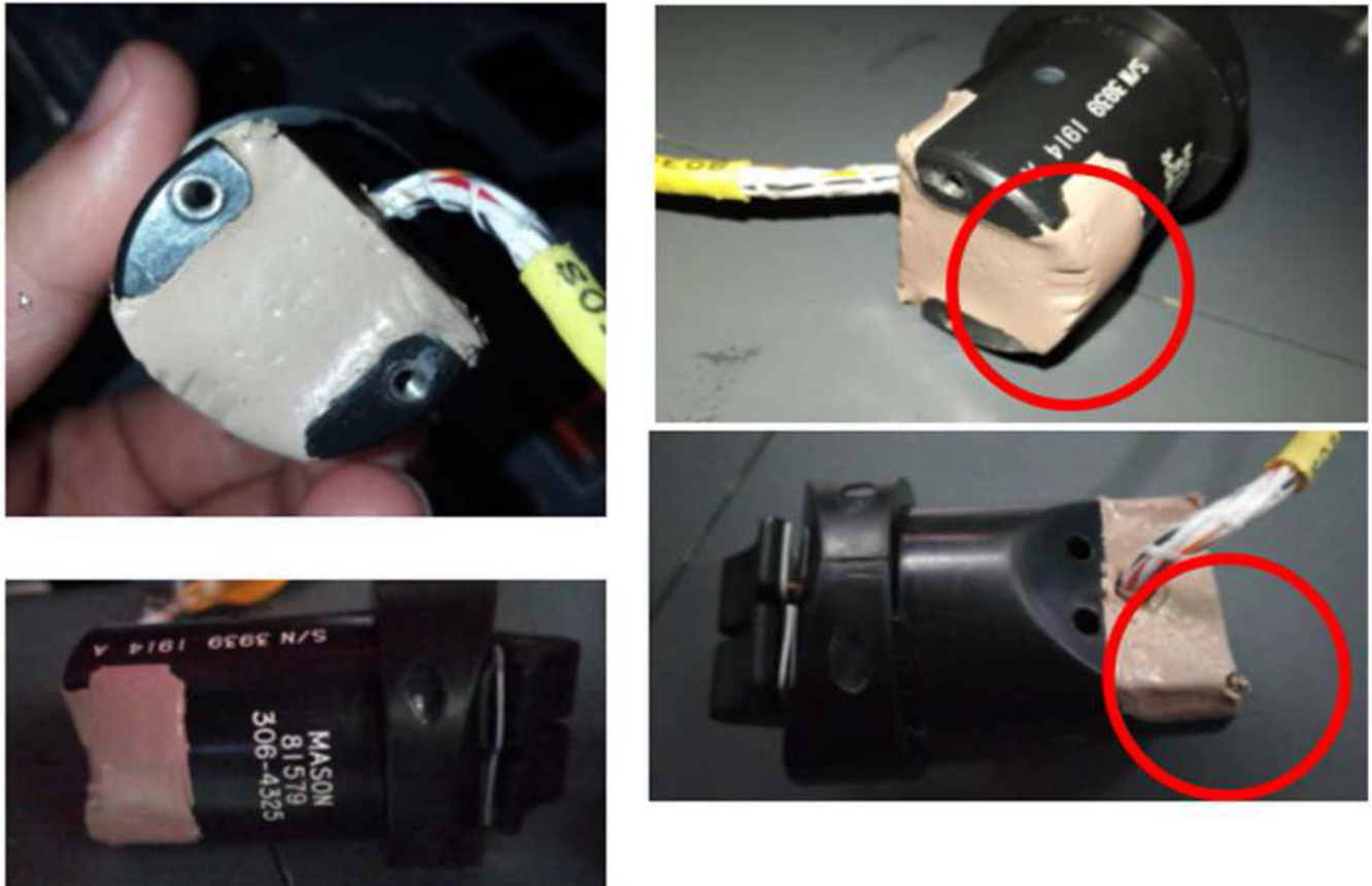
Figure 3. Captain-side pitch trim control switch after removal from the incident airplane (Source: Republic Airways).
