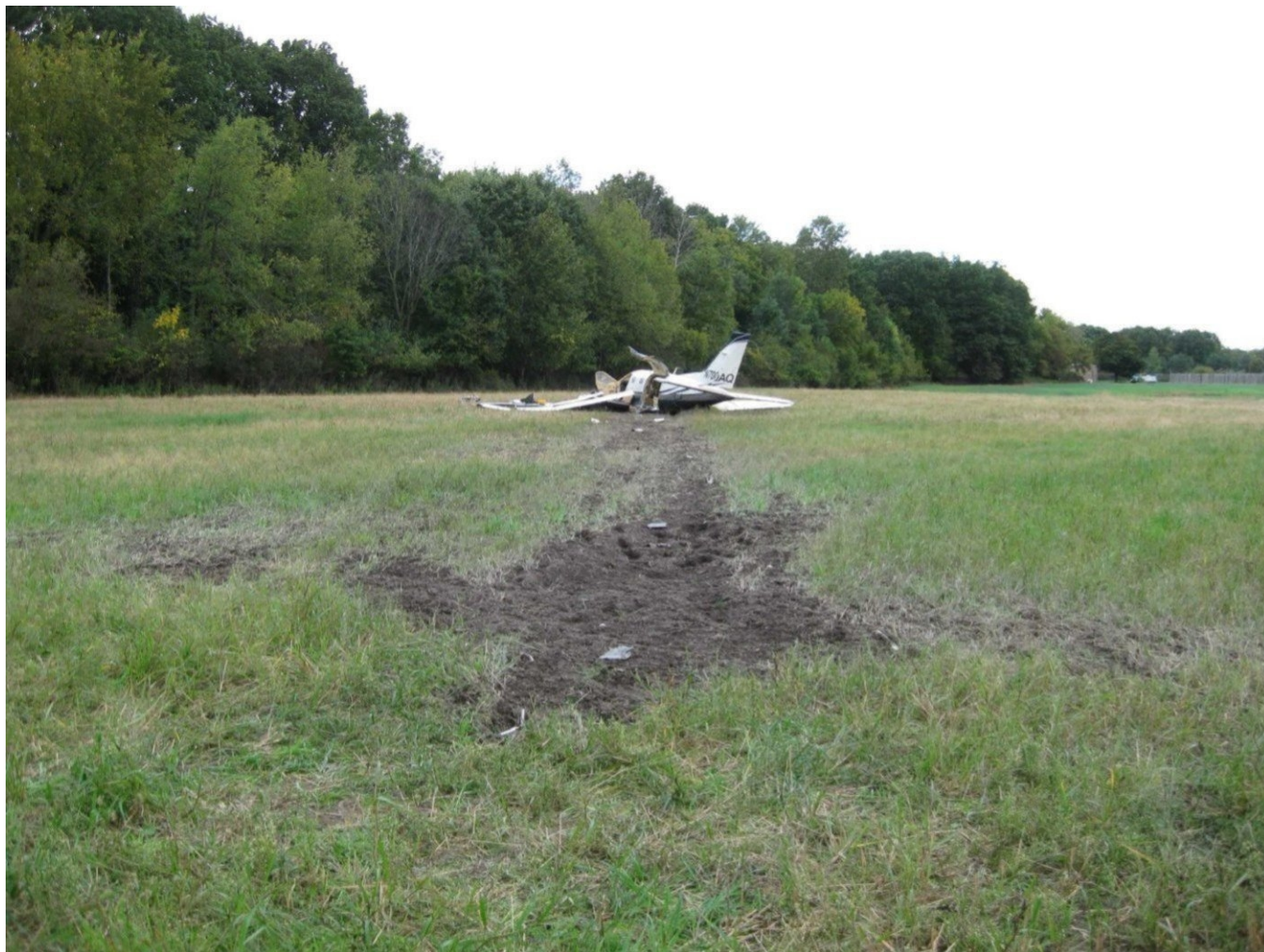
Figure 5. Initial impact point and ground scar.
