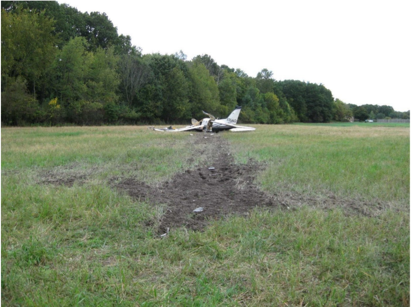
Figure 5. Initial impact point and ground scar.
