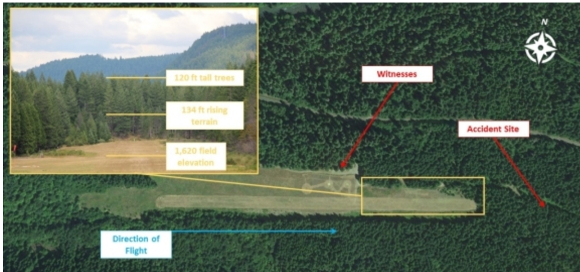
Figure 2: Terrain Elevations along Flight Path
