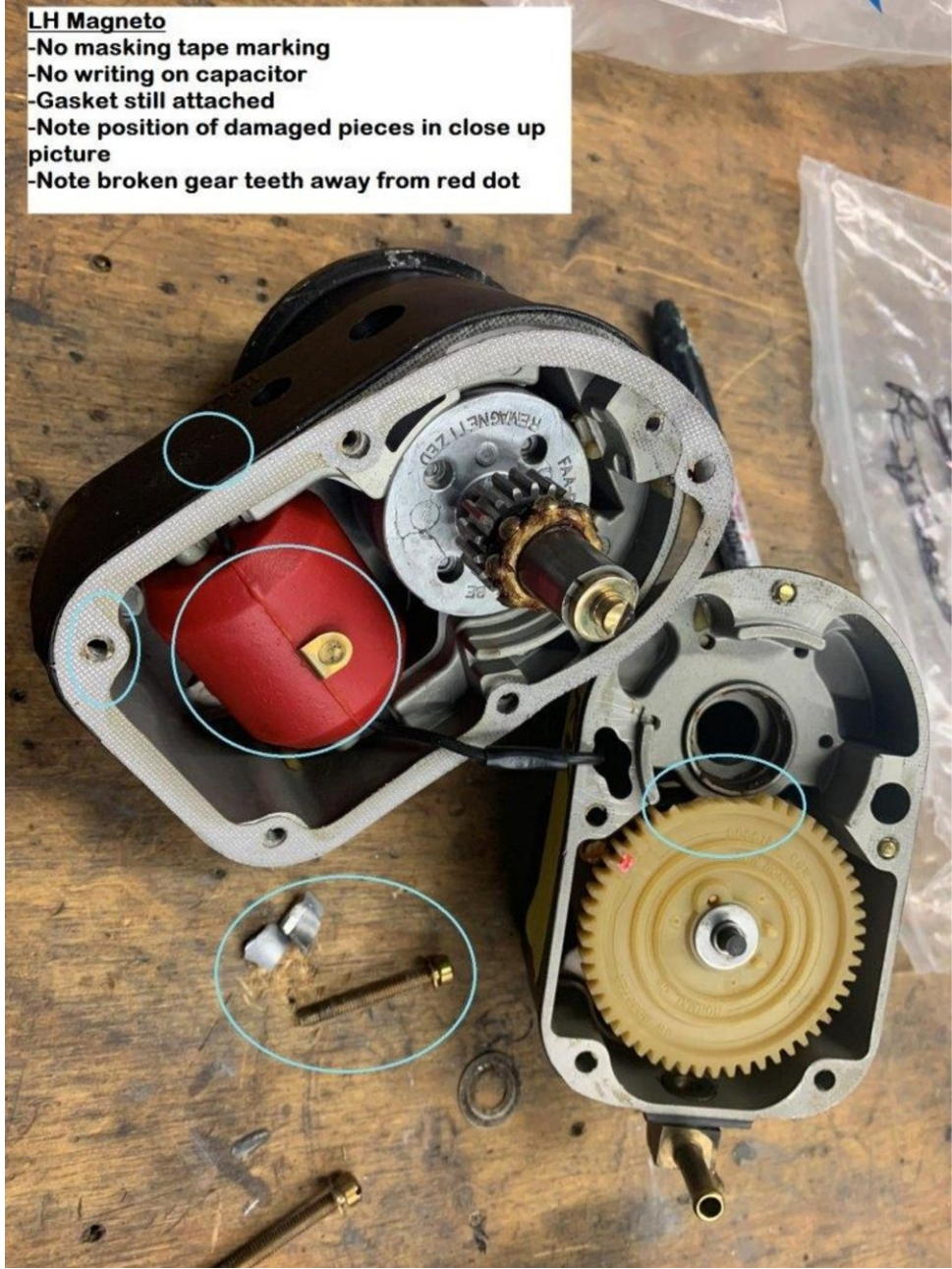
Figure 4. View of Left Magneto During Disassembly (courtesy Myers Aviation)
