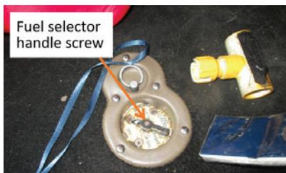
**Figure 3.** Photograph of fuel selector. (Source: FAA)
