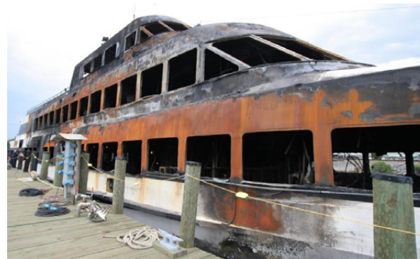
Figure 22. Exterior damage to the Spirit of Norfolk , starboard side
