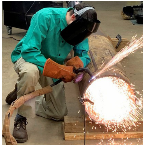
Figure 35. Michael Meadows, materials engineer in the Materials Laboratory Division, uses a plasma torch to cut samples from a section of cracked pipe.
