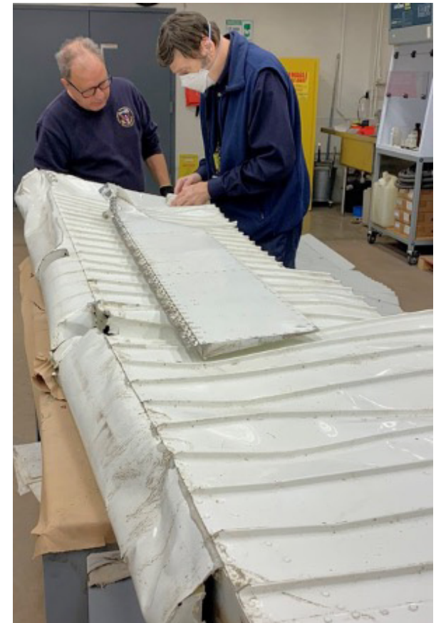
Figure 36. Edward Komarnicki, laboratory technician, and Frank Zakar, materials engineer, both in the Materials Laboratory Division, examine a portion of the horizontal stabilizer from the wreckage of a de Havilland DHC-3.
