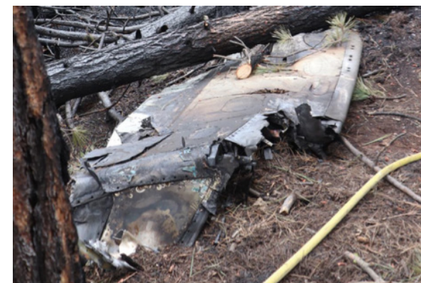
Figure 9. The left wing, winglet, and aileron of the destroyed airplane. The plane caught fire in the accident, and the wreckage was scattered across a wooded area.
