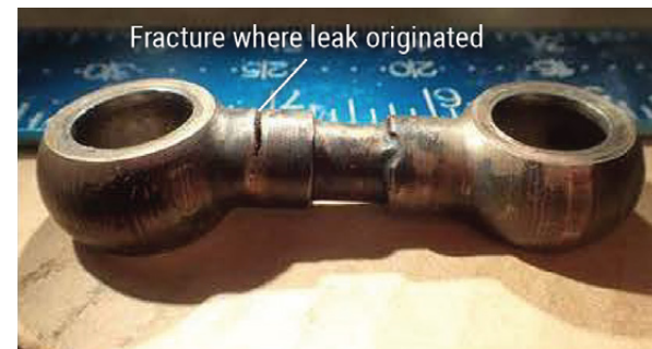
Figure 20. The fractured banjo tube from the Endo Breeze . SOURCE: QC METALLURGICAL, INC.
