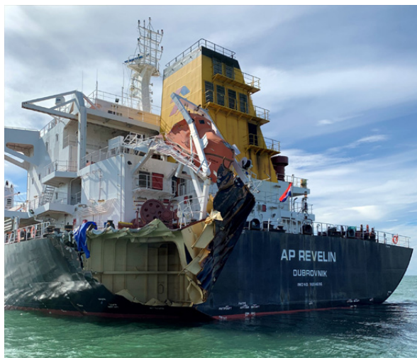
Figure 24. Damaged stern area of the AP Revelin after the collision.
