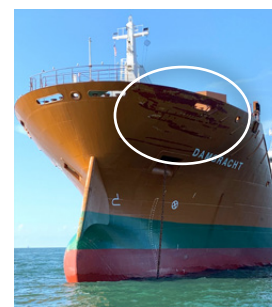
Figure 25. Port bow of the Damgracht after the collision, with damage circled in white.
