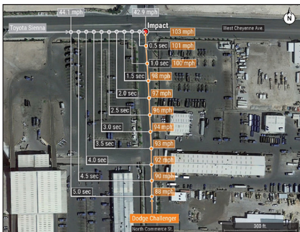
Figure 17. Relative positions and speeds of the Dodge and Toyota leading up to the North Las Vegas, Nevada, crash events.
