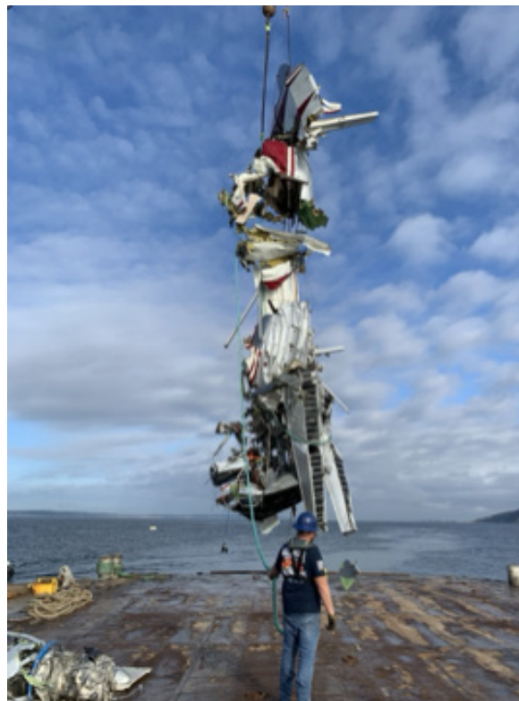
Figure 6. The mangled left wing, winglet, and aileron of the de Havilland DHC-3, post crash.
