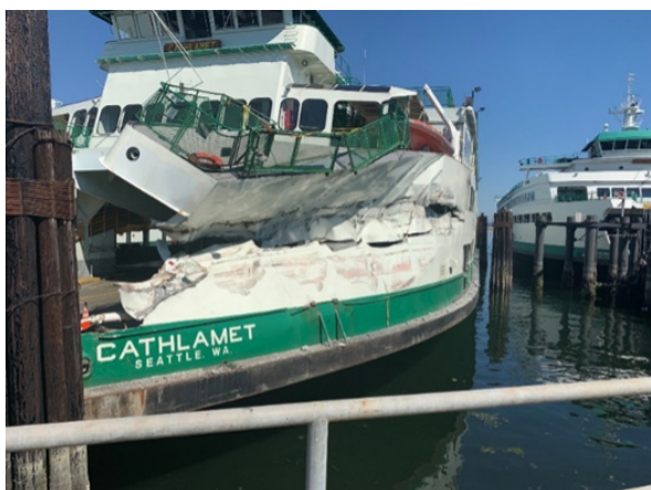
Figure 23. The damaged Cathlamet after the contact with the dolphin.
