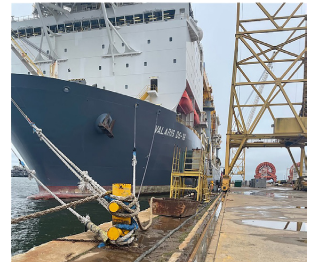
Figure 27. VALARIS DS-16 moored at STEHMO Shipyard at an unknown date before the casualty, with lines secured to bollard 6 (before lines were adjusted for the March 12 strong winds).
