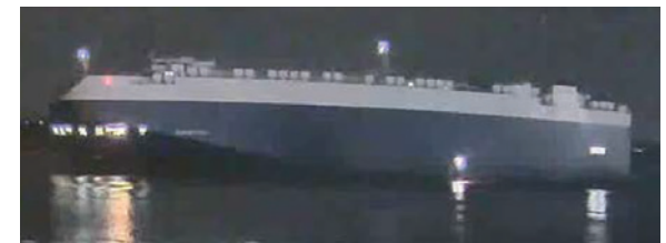
Figure 4. The Golden Ray departing Jacksonville, Florida, about 0130 on September 7. The light amidship is the open portside pilot door. (The lights on the blue hull at the bow and stern are mooring line stations.)
