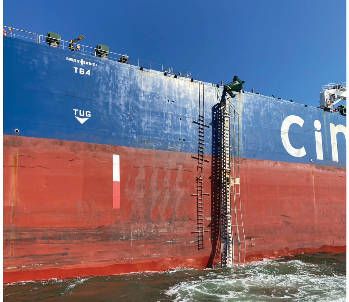
Figure 45. The Atina 's damaged accommodation ladder. SOURCE: COAST GUARD
