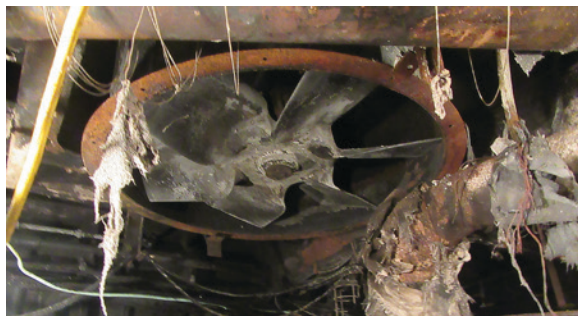
Figure 105. Starboard exhaust trunk fan (post-fire) located above the No. 1 generator. SOURCE: COAST GUARD
