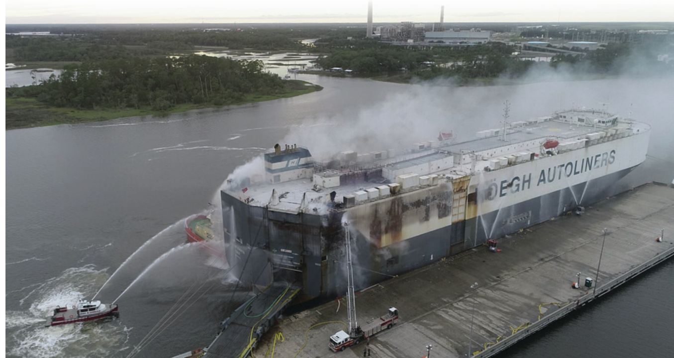
Figure 96. Firefighters conducting exterior boundary-cooling the day after the fire was discovered. SOURCE: JACKSONVILLE FIRE AND RESCUE DEPARTMENT
