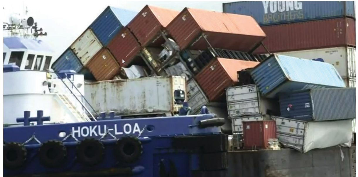
Figure 156. The collapsed row of containers, from the starboard quarter of the Ho'omaka Hou . SOURCE: COAST GUARD
