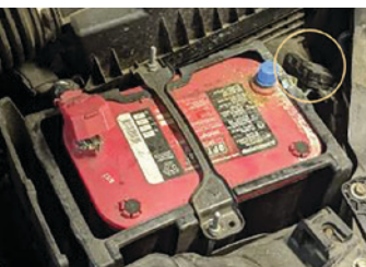
Figure 103. Excerpt from Grimaldi battery disconnect procedure showing a vehicle battery secured with a blue plastic negative terminal cap and disconnected cable (circled) tucked inside. SOURCE: GRIMALDI
