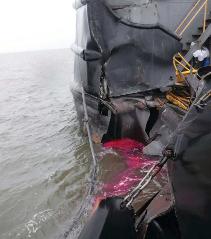
Figure 25. The port side of the Cheramie Bo Truc No 22 , post-collision, showing the compromised no. 1 port fuel tank and oil spillage. SOURCE: COAST GUARD.
