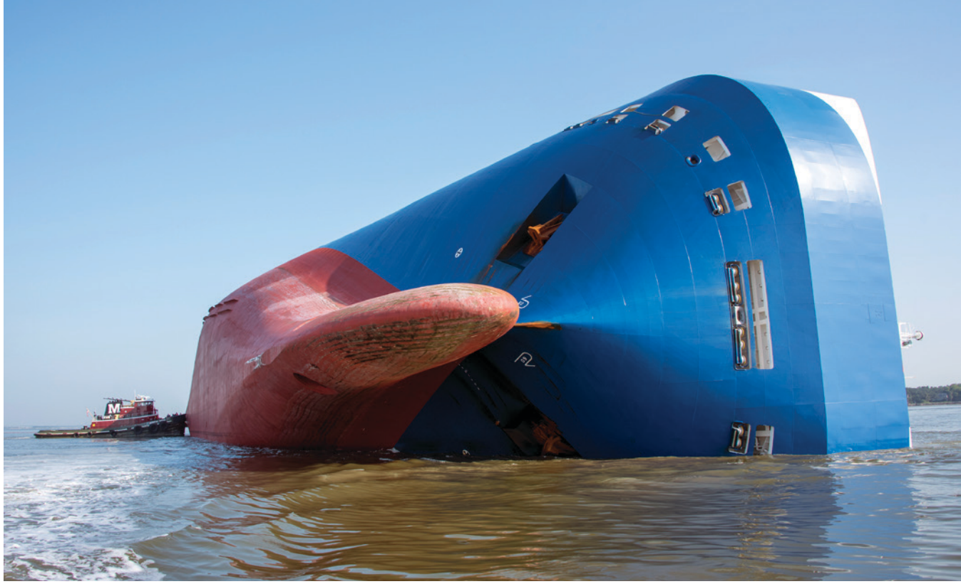
Figure 2. The Golden Ray heeled to its port side. SOURCE: COAST GUARD
