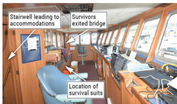
Figure 14. Photo of the bridge of the Scandies Rose taken from the starboard helm station.
