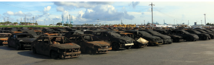
Figure 95. Thermally damaged vehicles after removal from the Höegh Xiamen , Blount Island, Jacksonville, Florida, July 23, 2020.
