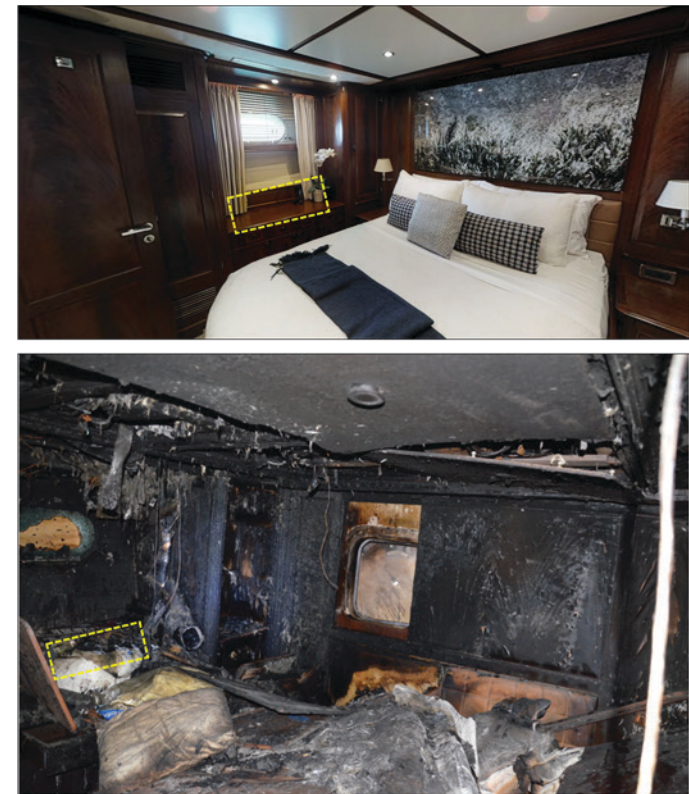
Figure 88. Promotional and postaccident photos indicate location of the candles (yellow rectangle) in the unattended port VIP suite. SOURCE [TOP PHOTO]: MCA YACHTS
