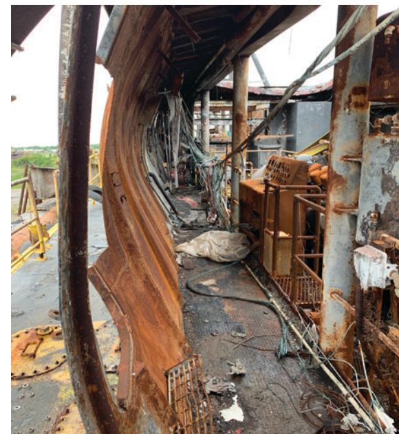
Figure 138. Post-salvage images of the Waymon Boyd lever room and captain's office (above) and engine room portside bulkhead, bowed outward (right).
