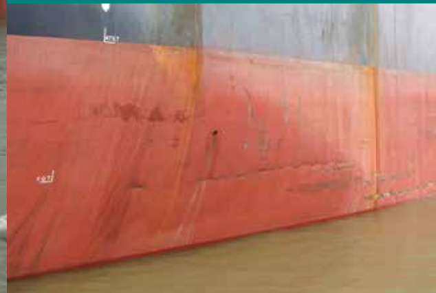
Damaged area of Anna Smile's hull. OPPOSITE PAGE, east tower of Louis Dreyfus grain elevator, which was damaged in the allision.
