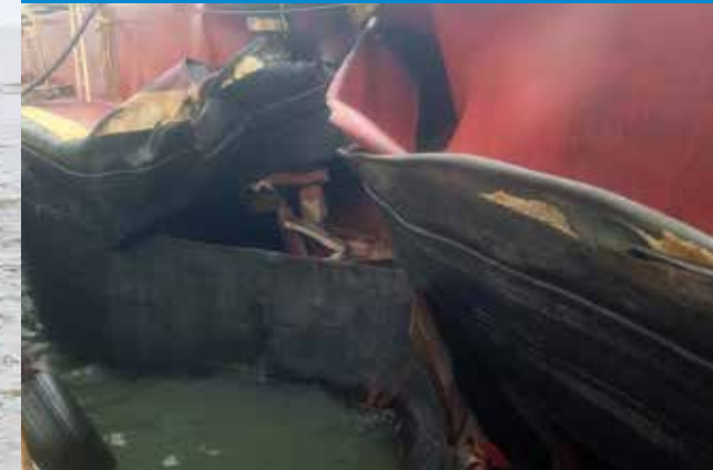
Bow damage of Summer Wind. ABOVE RIGHT, punctured hull on the starboard side of the lead barge in Miss Susan tow (photo by Coast Guard).
