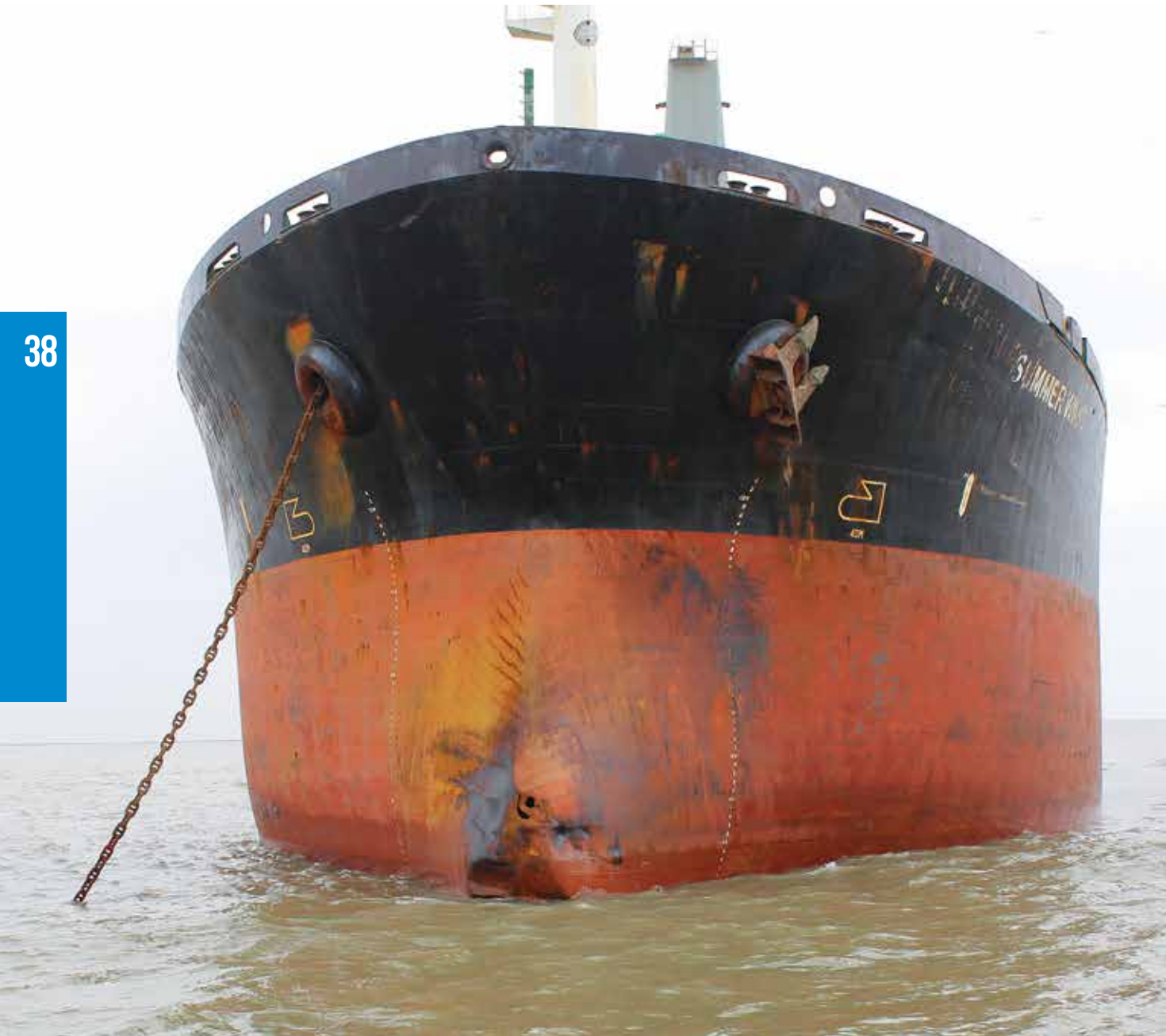
Bow damage of Summer Wind. ABOVE RIGHT, punctured hull on the starboard side of the lead barge in Miss Susan tow (photo by Coast Guard).
