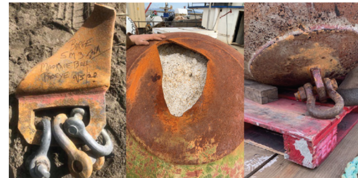
Figure 134. Left to right: SM-3 mooring buoy: failed weld (with three shackles) that separated from buoy; damaged top with padeye missing; and undamaged bottom padeye.
