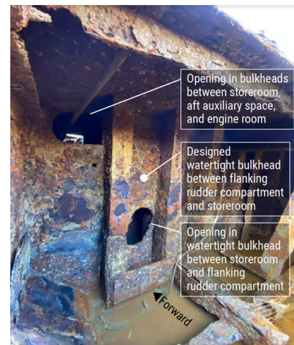
Figure 112. Flanking rudder compartment after recovery. Openings in bulkhead shown are also typical of other bulkheads below the main deck separating compartments. BACKGROUND SOURCE: COAST GUARD
