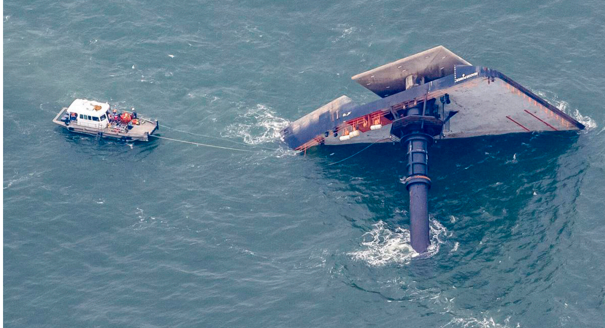
Figure 10. SEACOR Power after capsizing in the Gulf of Mexico when struck by severe thunderstorm winds.
