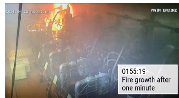
Figure 96. Top to bottom: CCTV screen captures of the main engine showing fuel spray in the area around the no. 5 cylinder the moment the fire started, and the progression ( time stamps are 4 hours ahead ). SOURCE: APL MARITIME
