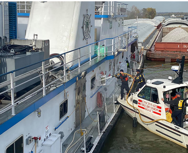
Figure 75. Firefighters deploying water into the engine room of the Capt. Kirby Dupuis through an open window.
