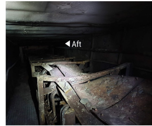
Figure 104. Left to right: Fire-damaged furnace and conveyor belt within the conveyor belt trunk above the furnace. SOURCE: COAST GUARD
