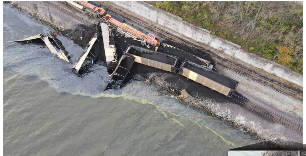
Figure 20. Drone view of the postcollision derailment of the two locomotives and eight hopper cars. Two additional hopper cars are submerged in the river. SOURCE: BNSF Inset: Location and close-up of the indentation from the forwardmost barge STC 3020 in the shoreline next to the railroad track. SOURCE: COAST GUARD
