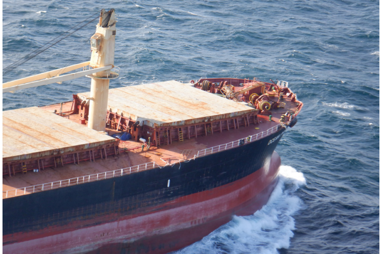
Figure 54. Knocked down mast and damaged bulwark, anchor windlass, and handrails on the Ocean Princess following the casualty. SOURCE: BUREAU OF SAFETY AND ENVIRONMENTAL ENFORCEMENT
