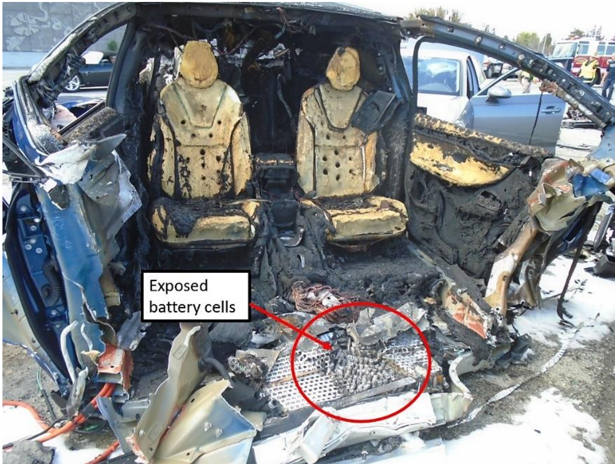
Figure 8. Interior view of the Tesla’s rear section, with exposed battery cells from the lithium-ion battery (circled in red) in the floorboard. (Source: CHP)
