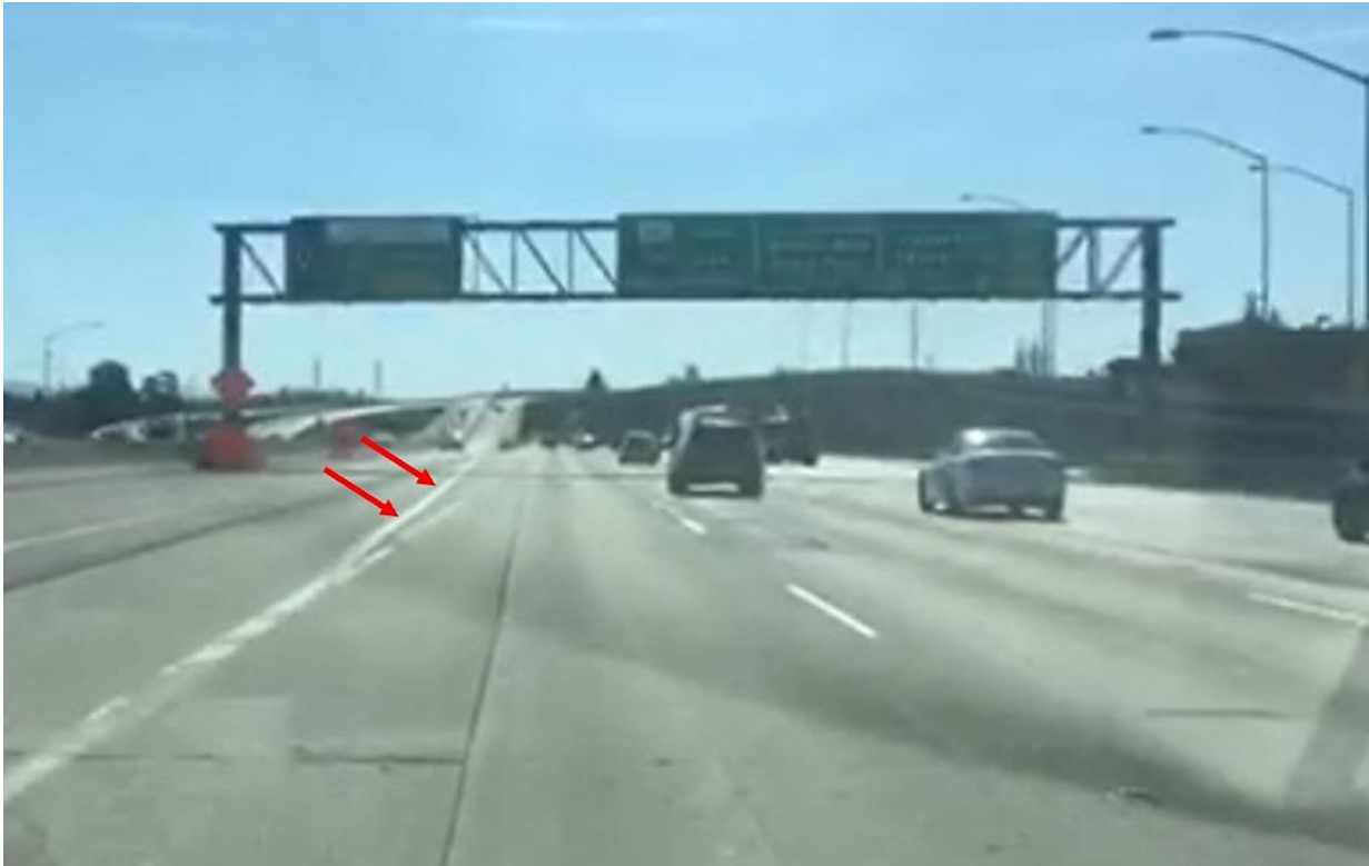
Figure 13. Southbound US-101 view from a video drive-through at 685 feet from crash attenuator. The 8-inch-wide solid white line marking the left side of the gore area (designated with red arrows) was more prominent and visible than the right side of the gore. (Source: NTSB video drive-through, March 27, 2018)
