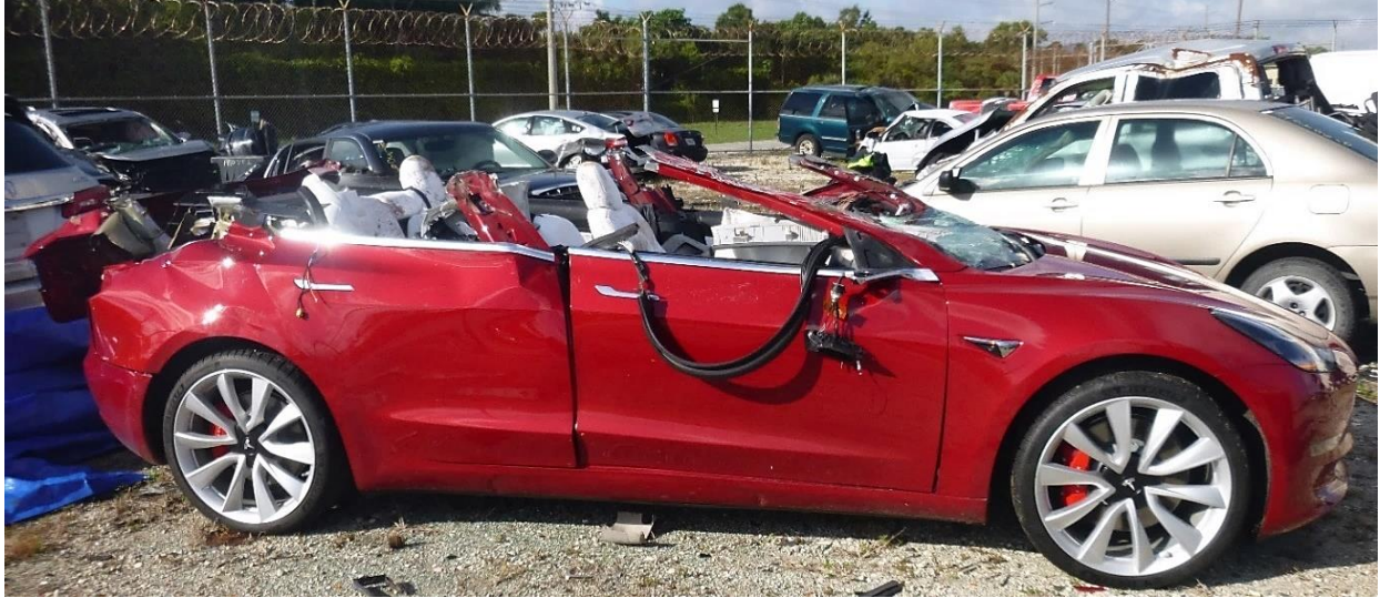
Figure 18. The 2018 Tesla after striking the side of a semitrailer in Delray Beach, Florida.
