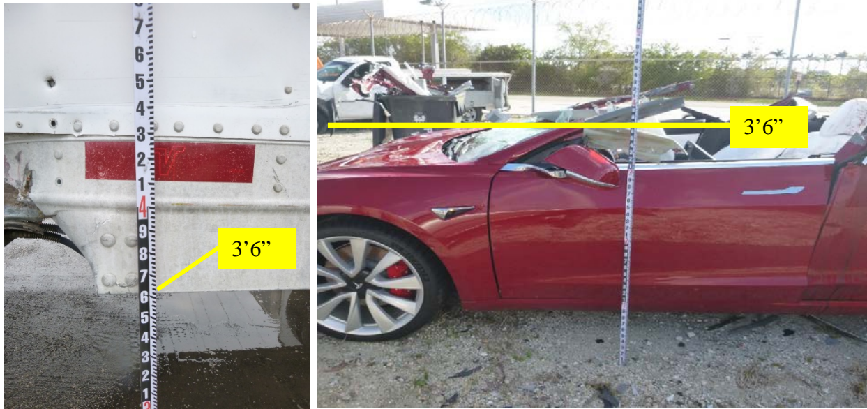
Figure 2 A-B - Photographs depicting the height of the lower edge of the trailer, measured at 3' 6" as shown in photo A and correlated to the damage to the passenger vehicle as shown by the yellow line in photo B.
