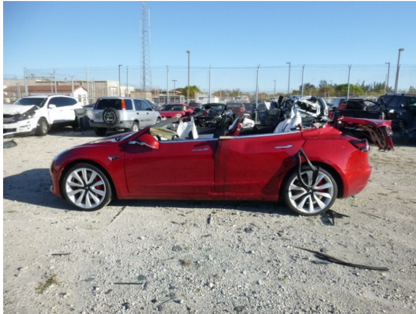
Figure 4 - Photograph depicting the left side view of the 2018 Tesla Model 3, showing collision damage and separation of the glass roof panel
