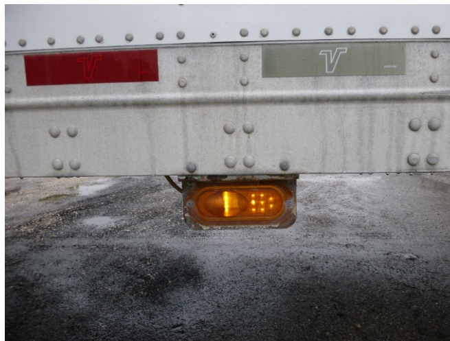
Figure 3 - Photograph depicting a view of the 2008 Vanguard semitrailer left side center amber marker light and red and white DOT C2 reflective retro reflective tape
