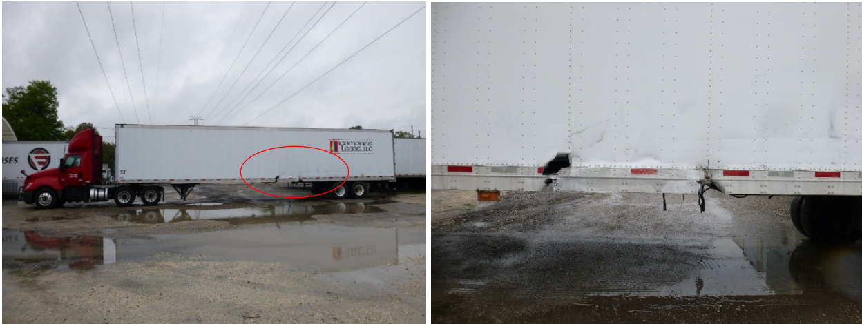
Figure 1 A-B - Photographs depicting the initial impact on the left side of the 2008 Vanguard semitrailer, area of impact circled in red, photo B is a focused view of the area of impact
