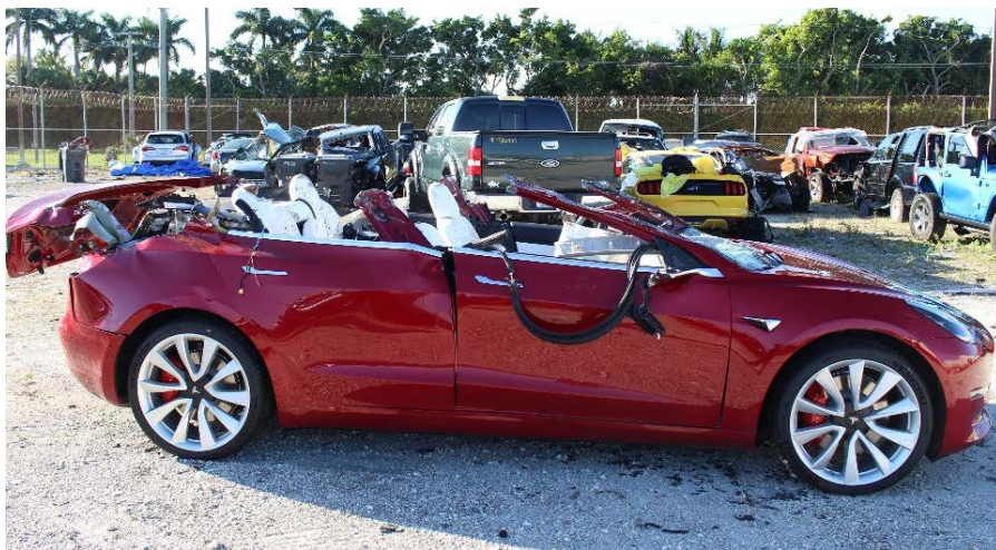
Figure 1: Photograph showing the Tesla Model 3 with extensive roof damage
