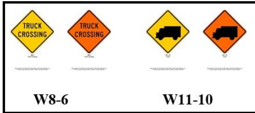
Figure 10 Illustration of the MUTCD “Truck Crossing” warning signs designated as W8-6 and W11-10.
