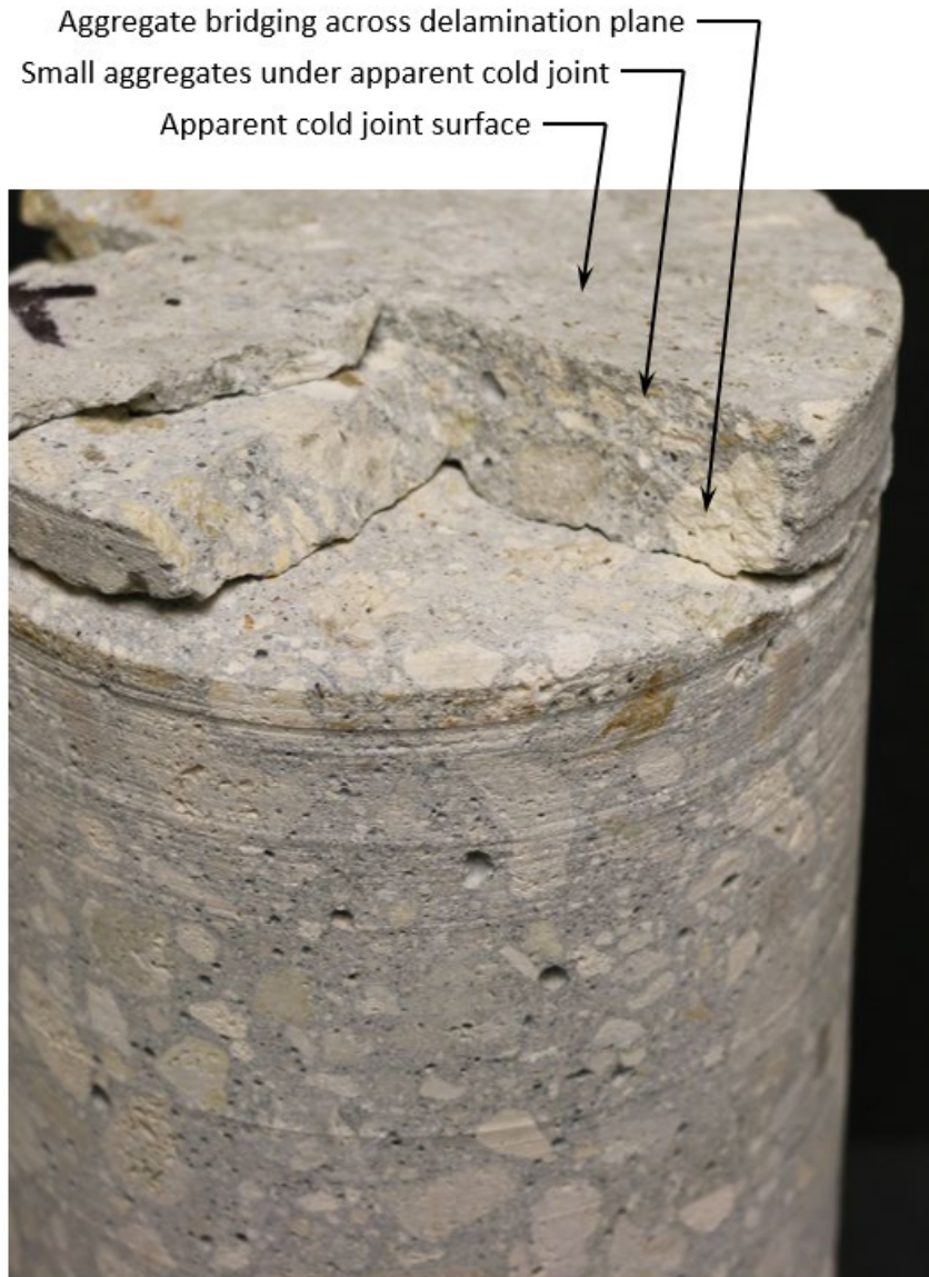
Figure 11. Annotated image of core extracted from south end of interface surface under Member 11.
