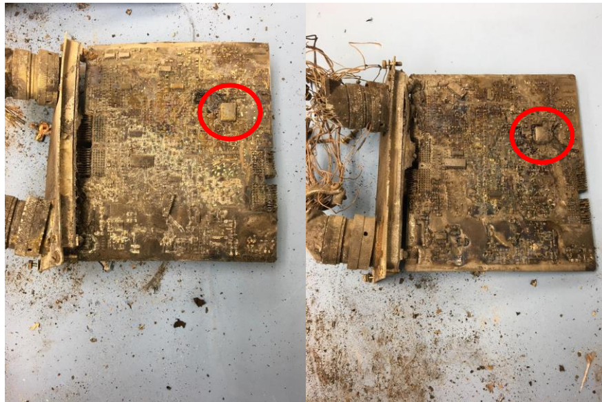
Figure 3. Photo of the unit's two internal boards after removal. The NVM chip is circled in red.
