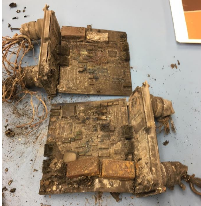
Figure 2. Photo of each lane of the VEMD after being removed and segregated.
