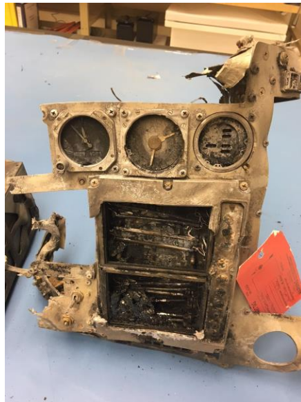
Figure 1. Photo of damaged unit with three other instruments still attached.
