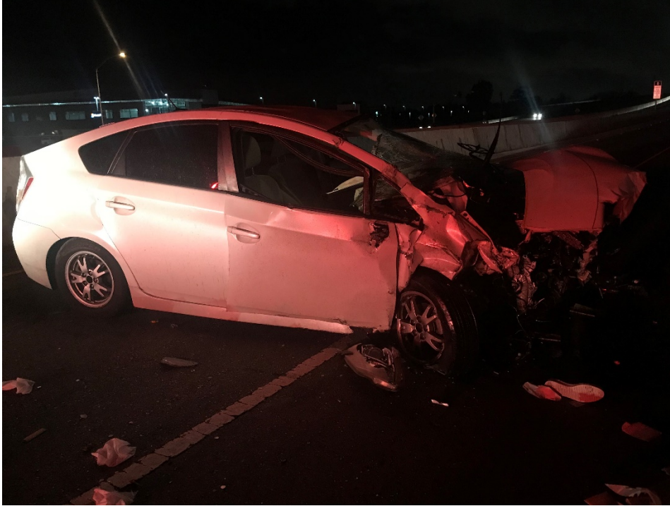
Figure 2. Photo showing right front-end damage to Toyota Prius at scene of collision with crash attenuator on March 12, 2018 – eleven days prior to fatal March 23 rd crash at same location.
