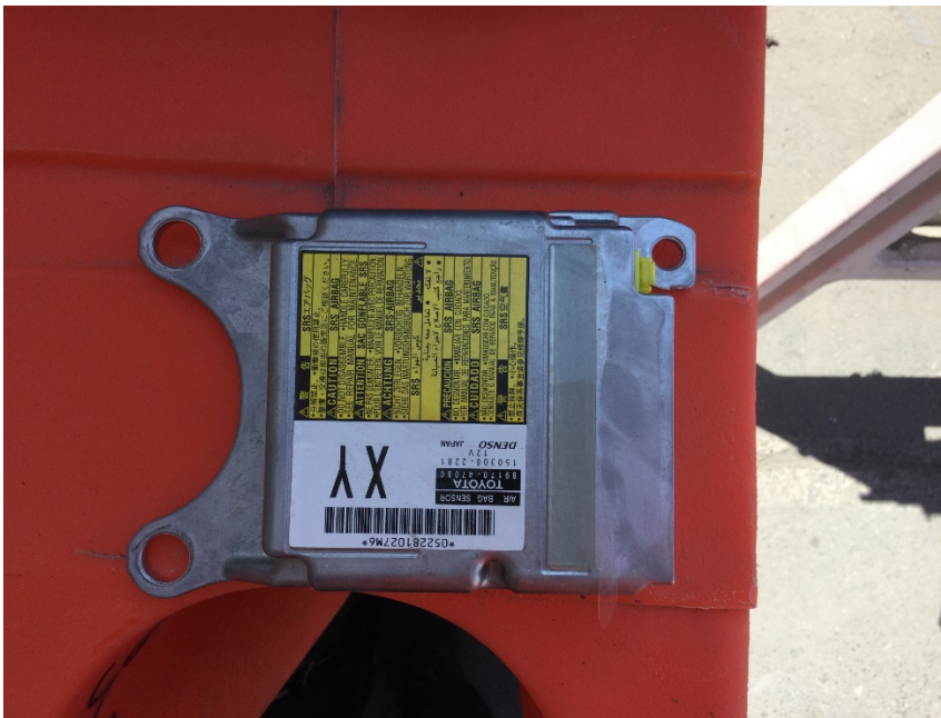
Figure 5. Photo showing the location of the airbag control module after it was removed from the Toyota Prius during inspection of vehicle at impound facility on August 1, 2018.
