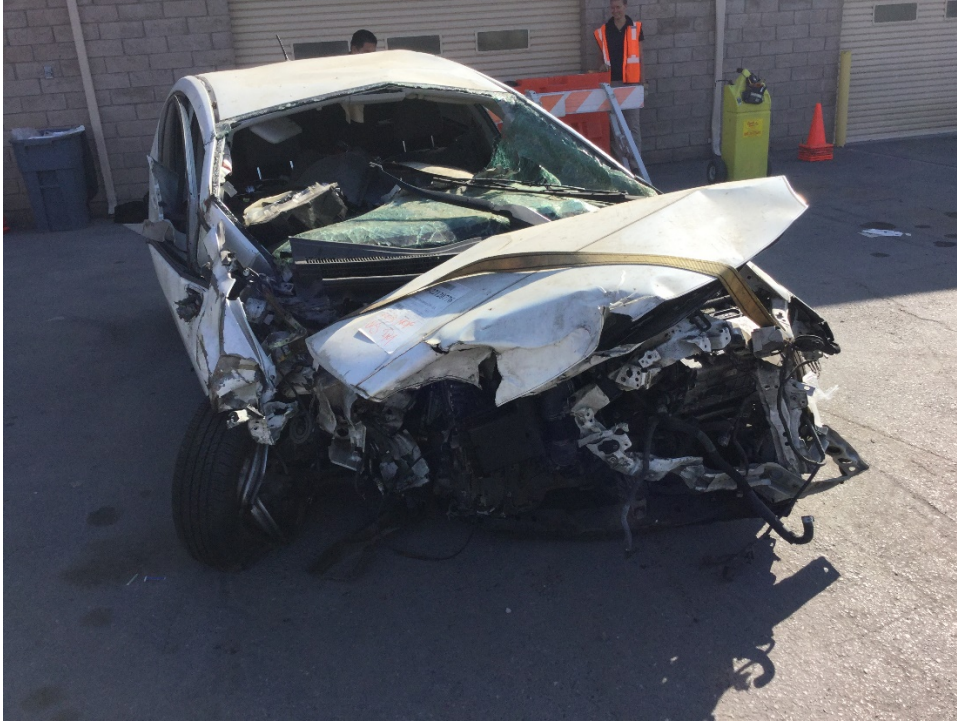
Figure 3. Photo showing front-end damage to Toyota Prius during inspection of vehicle at impound facility on August 1, 2018.
