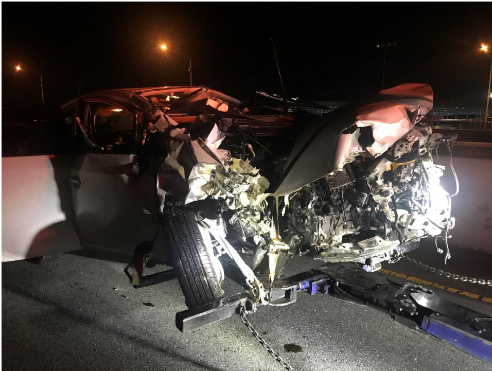
Figure 1. Photo showing front end damage to Toyota Prius at scene of collision with crash attenuator on March 12, 2018 – eleven days prior to fatal March 23 rd crash at same location.
