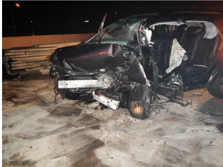
Figure 2 – Postcrash photo of 2008 Lexus SUV on November 14, 2015, after colliding with non-operational crash cushion on US-101 southbound at the exit ramp transition to SR-85.
