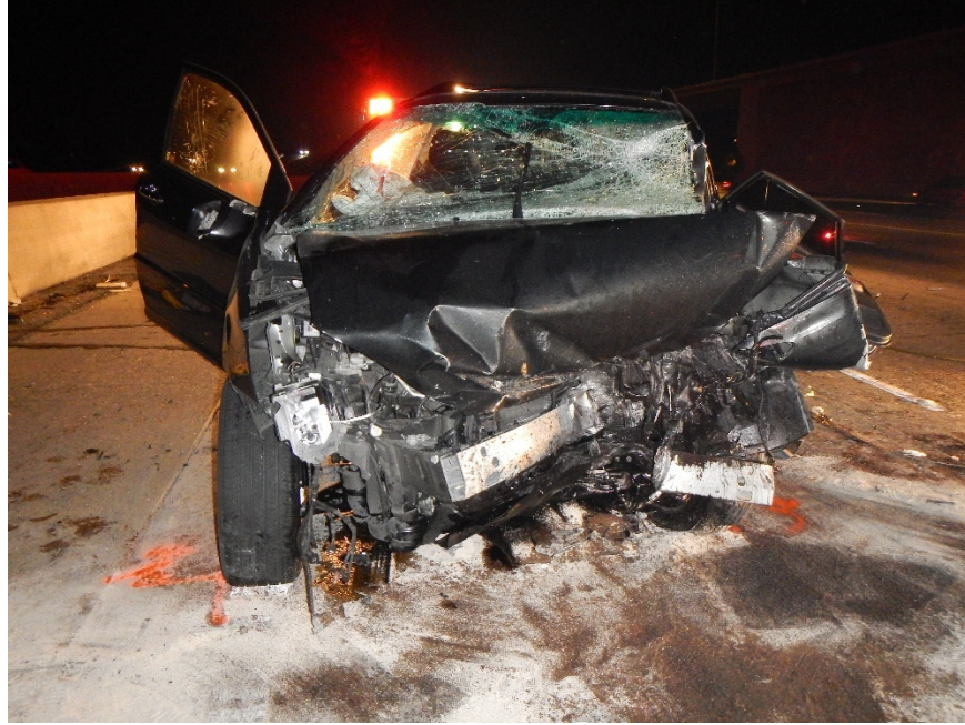
Figure 6 – Postcrash photo of 2008 Lexus SUV on November 14, 2015, after colliding with non-operational crash cushion on US-101 southbound at the exit ramp transition to SR-85.
