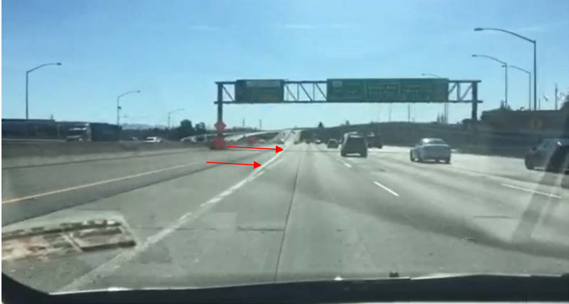
Figure 3E – Still image from video drive through at 685 feet from crash cushion. During the drive through the 8-inch wide solid white channelizing line (designated with red arrows) marking the left side of the gore area was the most prominent and visible.
