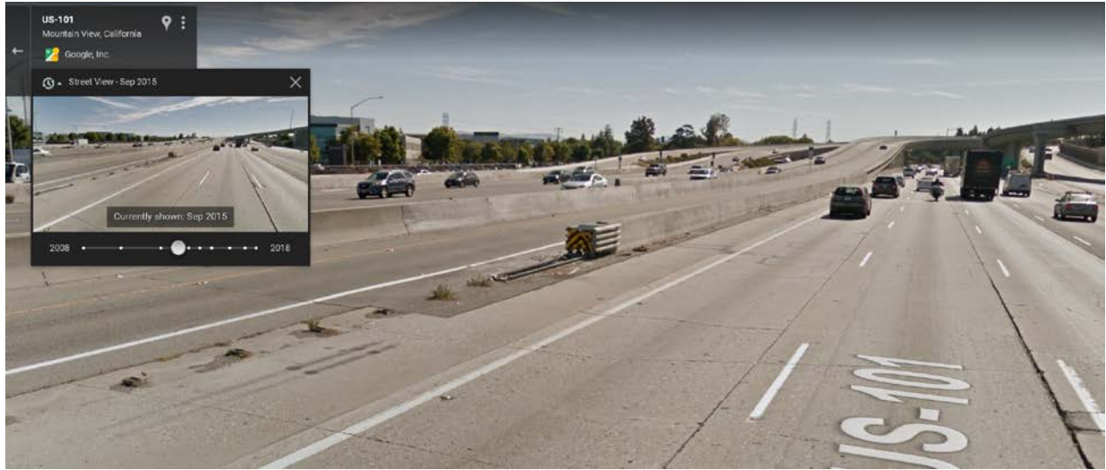
Figure 7C – Google Maps Street View image captured in September 2015 showing the crash cushion fully collapsed.
