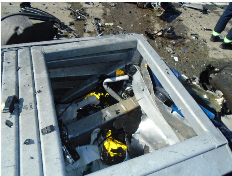
Figure 6D – Postcrash picture of damaged crash attenuator with Tesla vehicle components lodged inside of the hollow interior section of the crash cushion.
