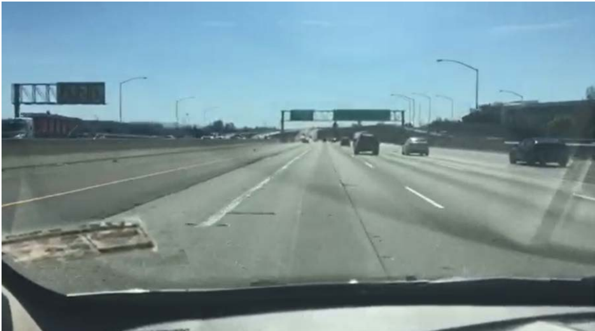
Figure 3D – Still image from video drive through at 950 feet from crash cushion. The beginning of the 8-inch wide solid white line can be seen in this image. Portions of the white line are faded with paint obliterated.
