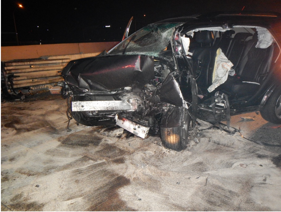
Figure 7A – Postcrash picture of 2008 Lexus SUV on November 14, 2015, after colliding with non-operational crash cushion on US-101 southbound at the exit ramp transition to SR-85.
