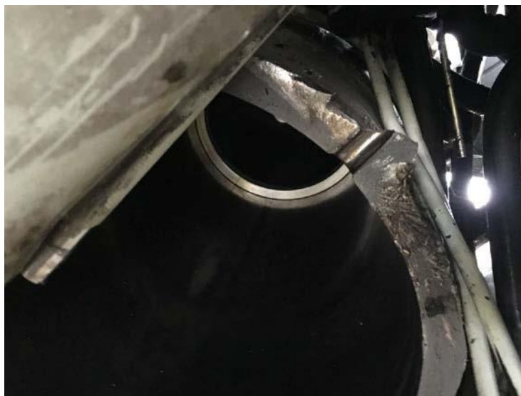
Fracture Surface on the Lower Section of the Left Main Landing Gear Cylinder
