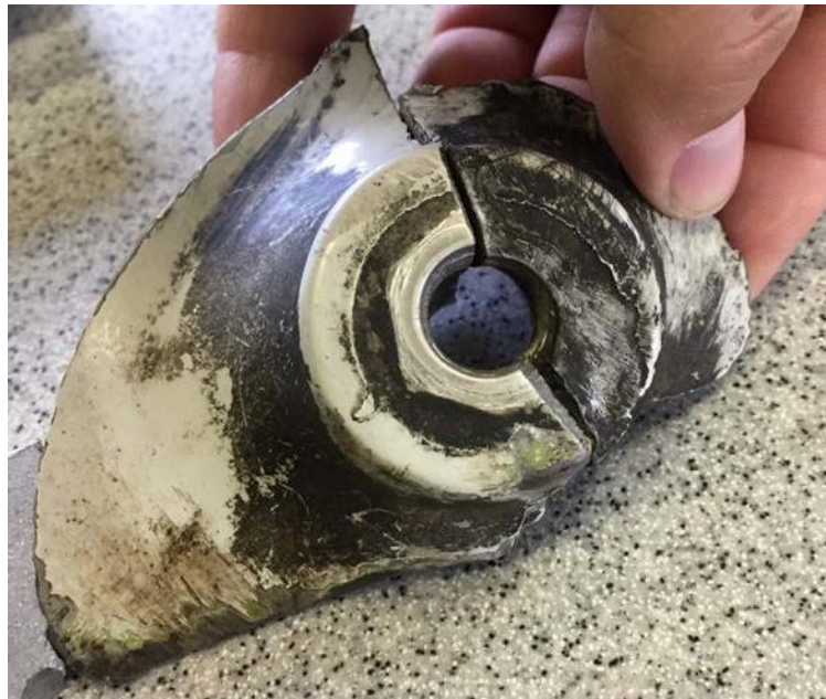
Air Fill Valve Bore Boss Pieces Recovered From Runway
