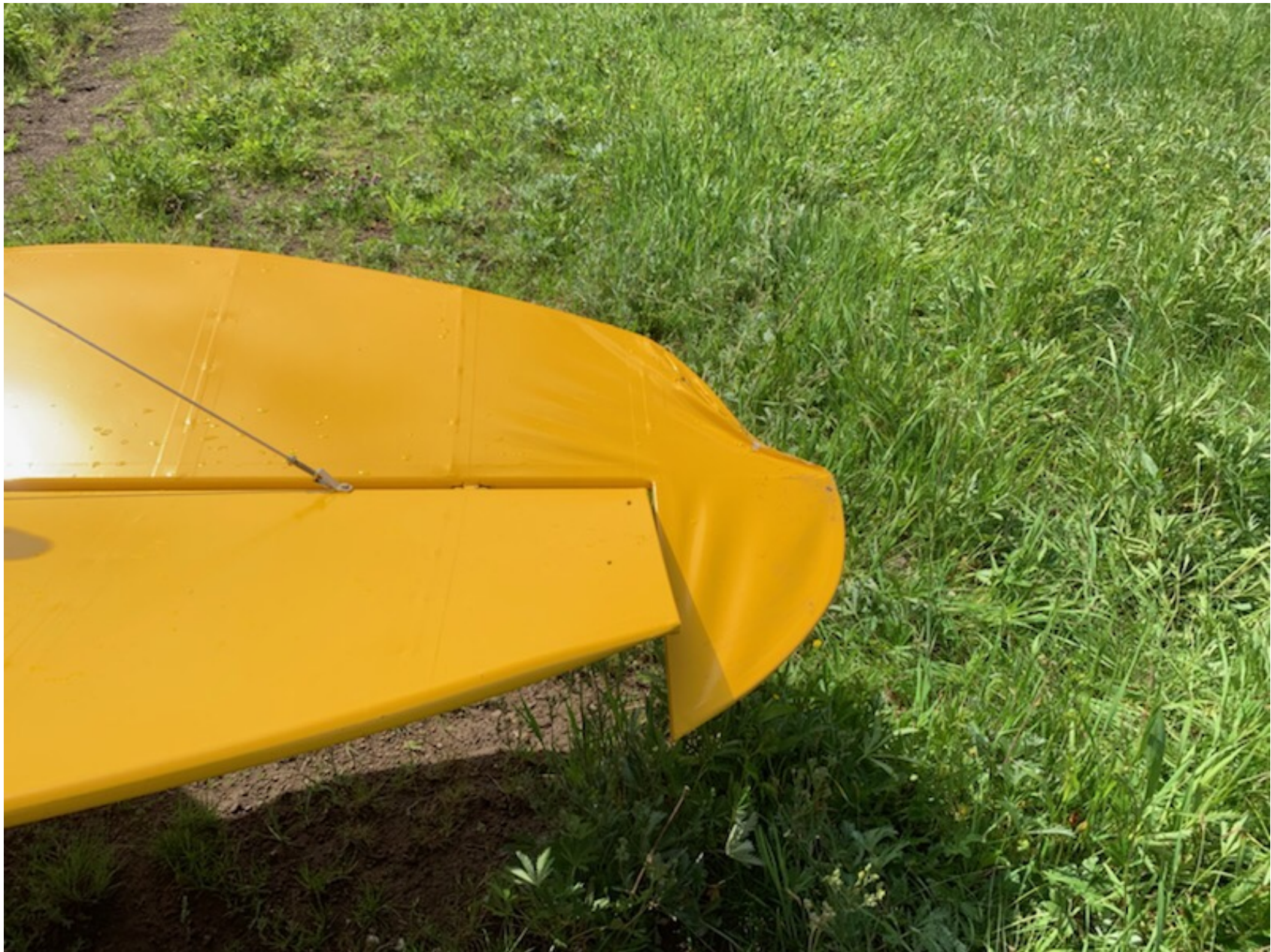
Photo 1 – View of damaged left elevator (courtesy of the pilot)
