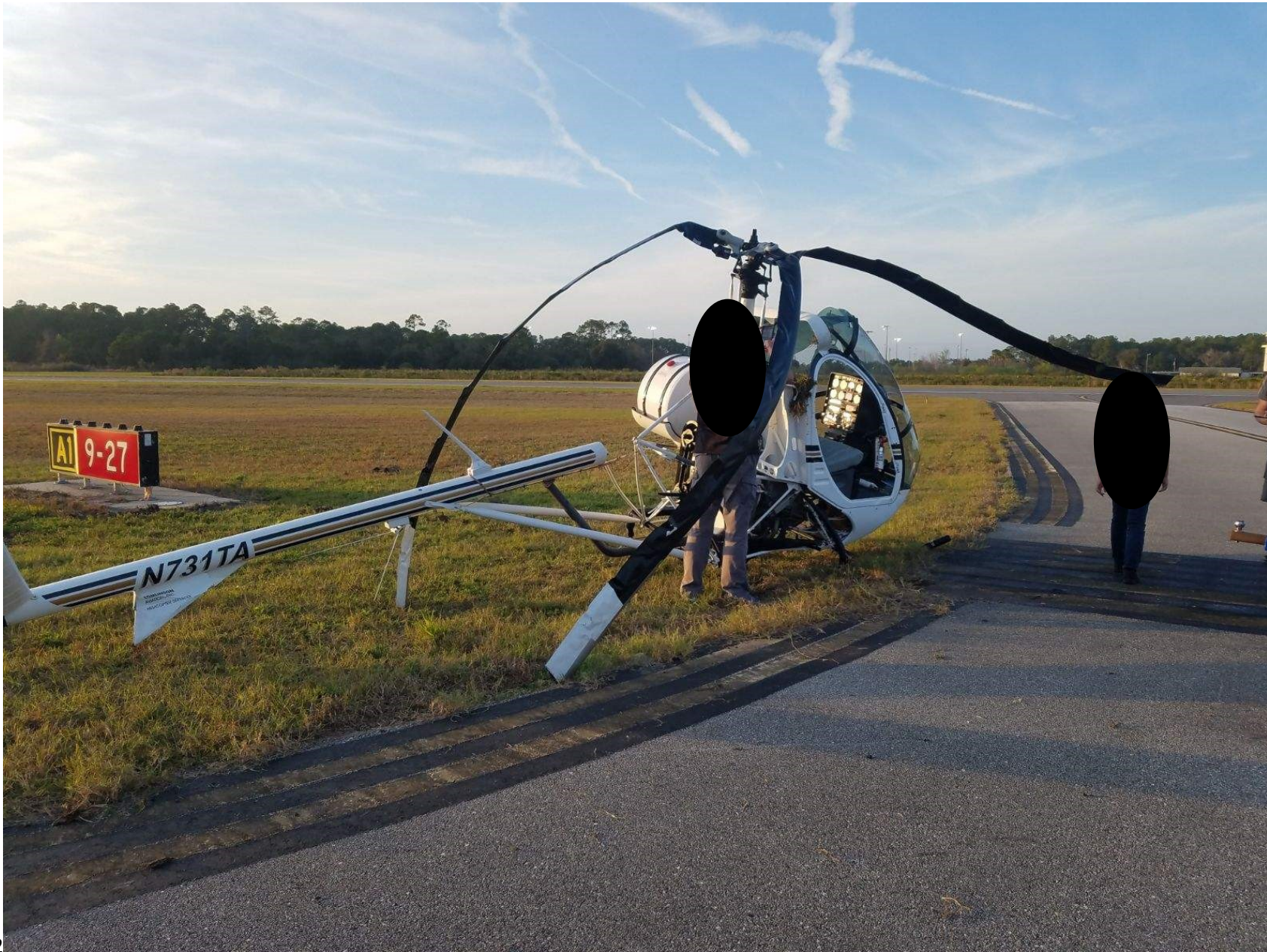
Photo 1 – View of main rotor and tailboom damage (photo courtesy of the FAA)
