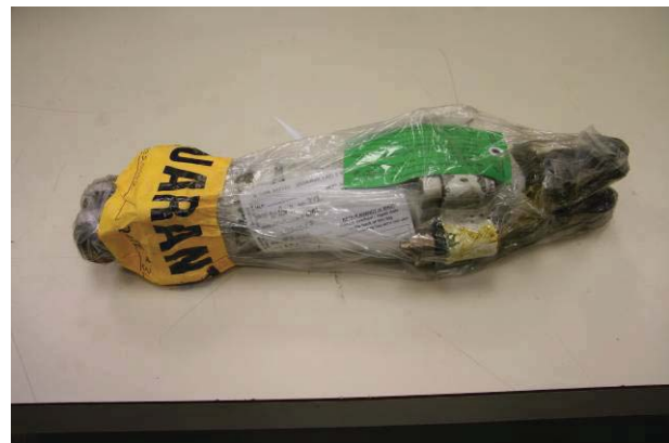
Figure 7: The 65-44610-4 NLG retract actuator removed from the box. The bag is sealed with “QUARANTINE” tape.
