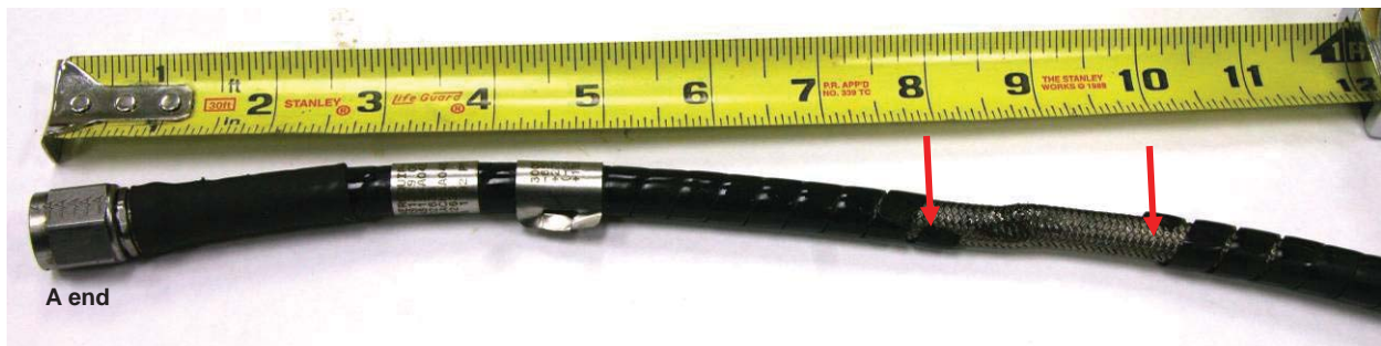
Figure 17: Missing spiral wrap.
