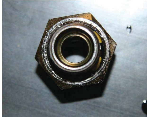
Figure 25: Union fitting installed in cap end.
