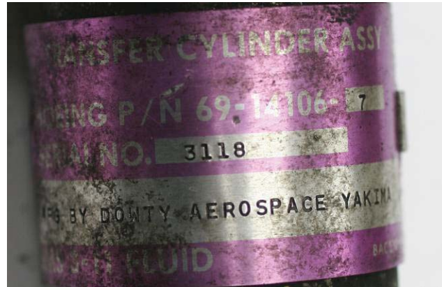
Figure 13: The identification tag for the transfer cylinder.
