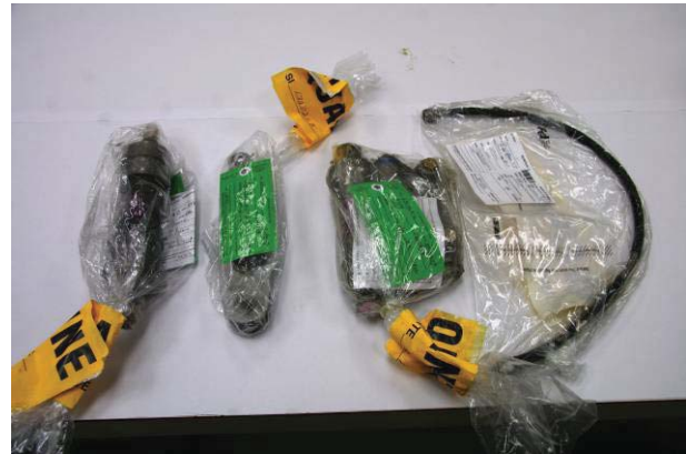
Figure 9: The contents of box #2, from left to right: the 69-14106-7 NLG transfer cylinder assembly, the 65C27360-5 NLG door operator crank assembly, the 65-44691-6 NLG modular package and the BACH8A04EE-0263S retract actuator hose.
