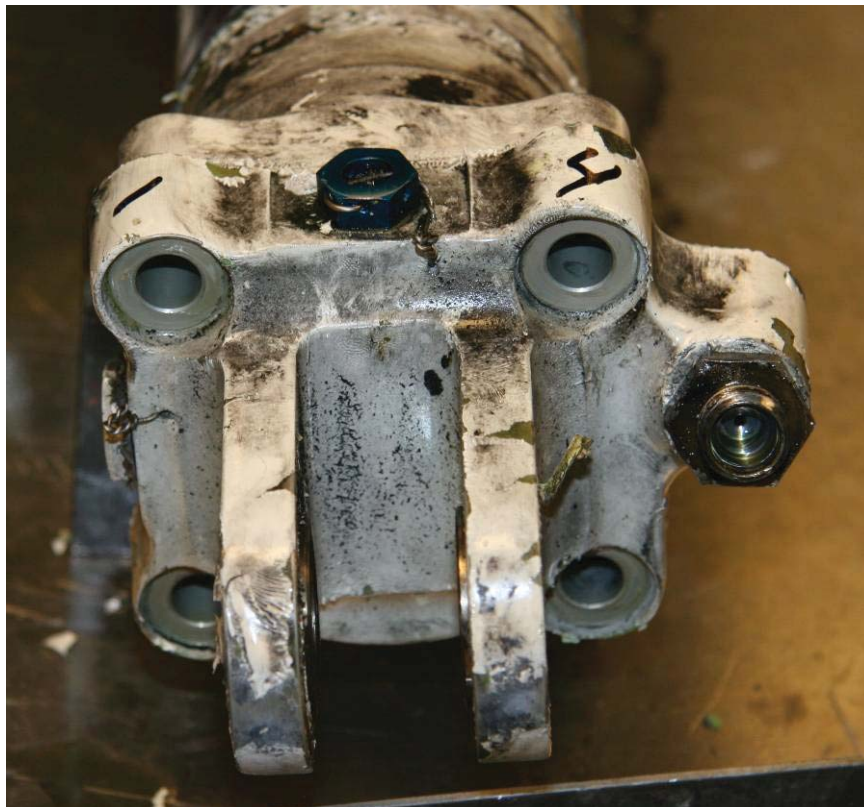
Figure 23: Bolts removed from head (item 4) end. Bolt locations are marked in counter-clockwise orientation.
