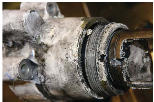
Figure 27: The bushing loosened from the cylinder.
