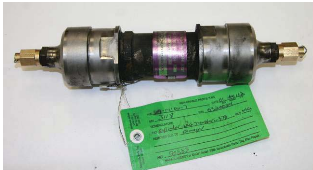
Figure 12: The 69-14106-7 transfer cylinder removed from the plastic bag.
