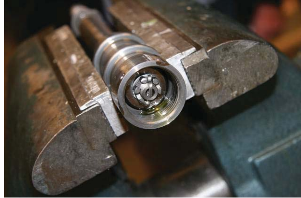
Figure 33: The sleeve retaining nut was removed.
