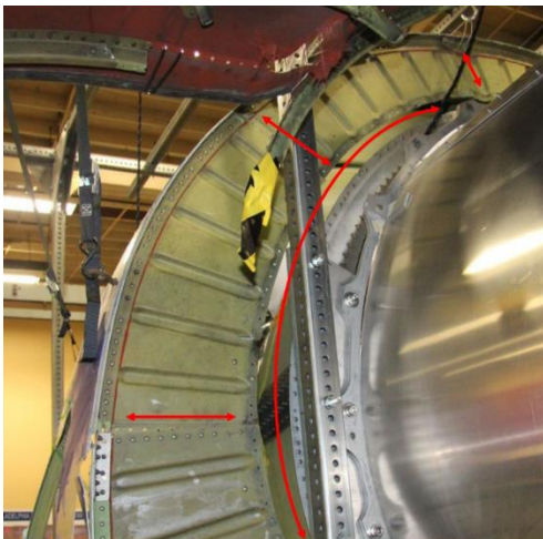
Figure 21 – Aft Bulkhead Joint Failure – Accident hardware Left Hand View (Aft Looking Forward)
