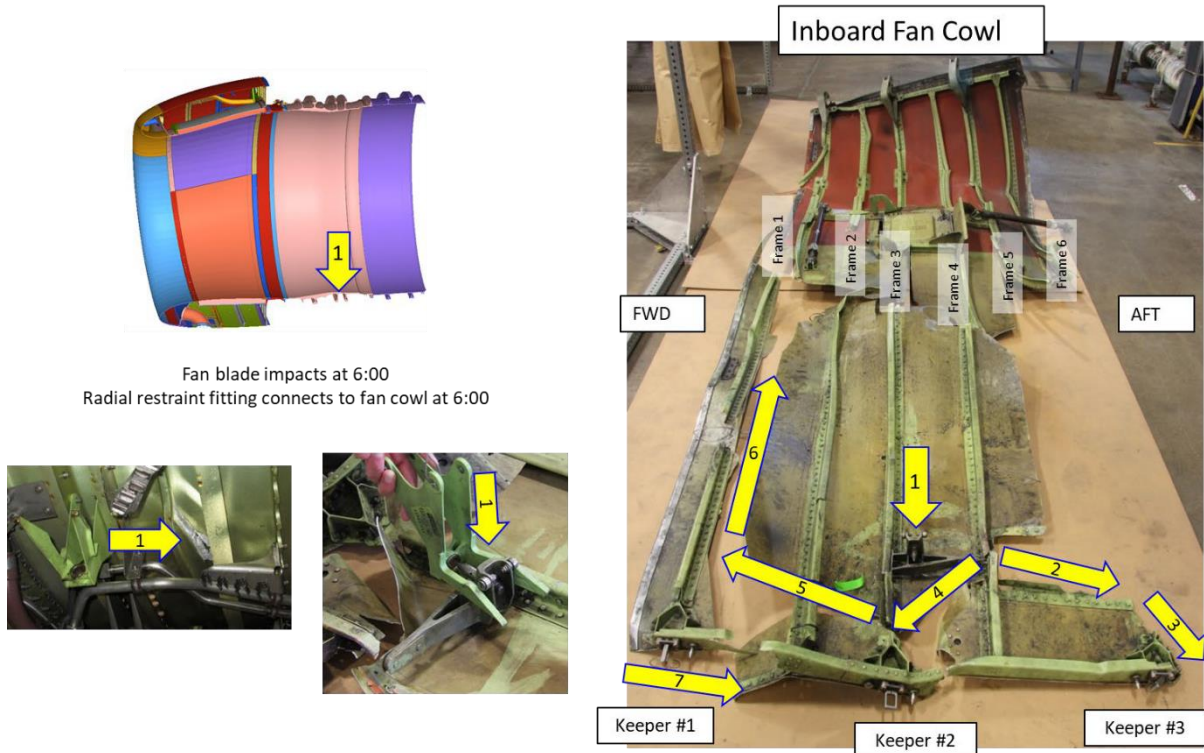
Figure 14 – Predicted Fan Cowl Failure Sequence
