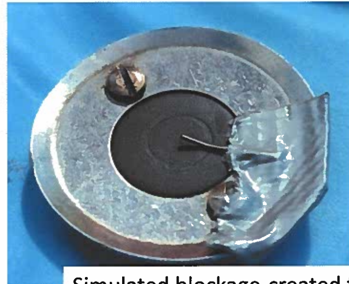
Simulated blockage-created for testing
