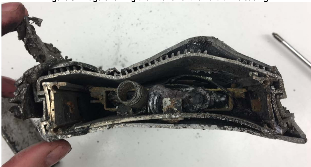
Figure 3. Image showing the interior of the hard drive casing.
