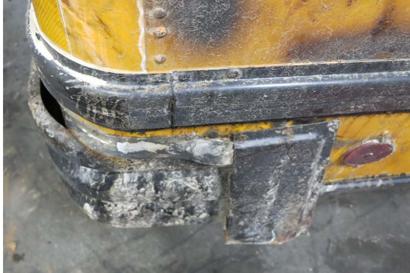
Figure 2: Damaged Right Rear Corner of Bus
