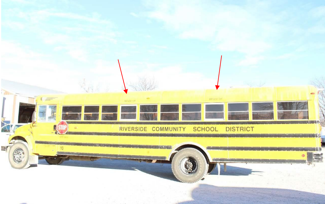
Photo #1: Exemplar school bus showing the location of the emergency exit windows.
