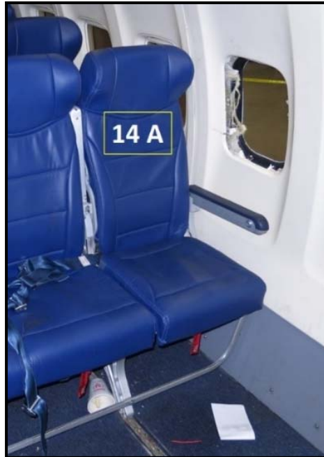
Photograph 1 – Row 14 ABC triple seat set showing seat 14A adjacent to broken window.
