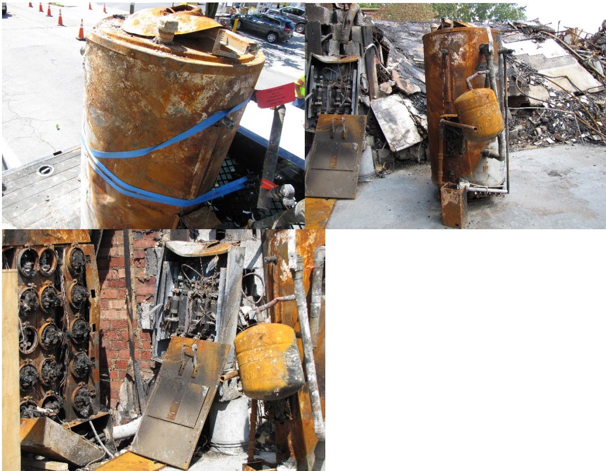
Figure 18: 8701 Arliss Street Silver Spring Apartment Building Water Heater, Electric Meters and Switch Box.
