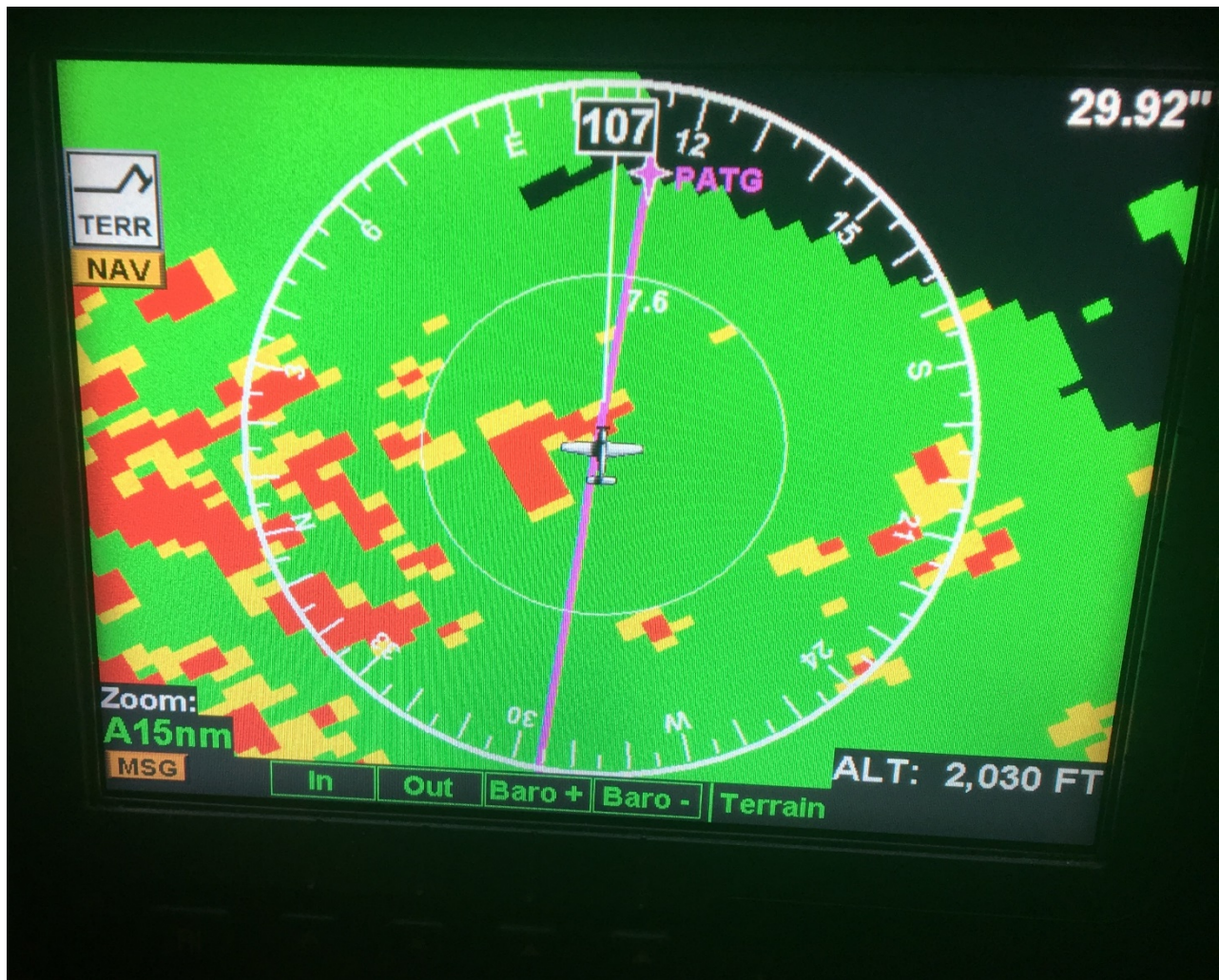
Photo 5. Garmin MX20 display – Terrain mode.
