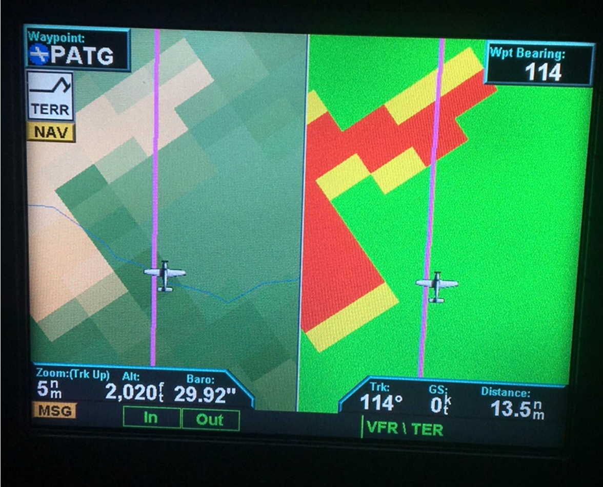
Photo 6. Garmin MX20 display – Split mode.
