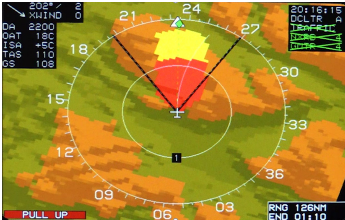
Figure 6. An example of how the Chelton EFIS software version 6.0B depicts TAWS cautions (yellow) and warnings (red) on the MFD.
