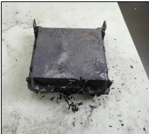
Figure 2. BNSF 3967's certified crashworthy event recorder memory module
