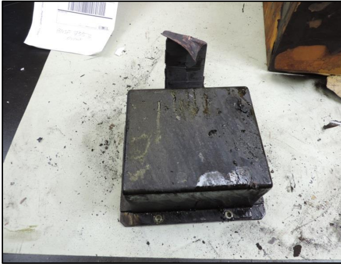
Figure 10. BNSF 7553's certified crashworthy event recorder memory module
