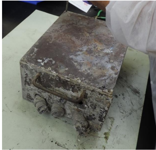
Figure 1. BNSF 3967's locomotive event recorder as received
