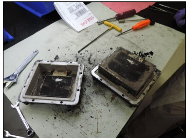
Figure 3. BNSF 3967's certified crashworthy event recorder memory module opened
