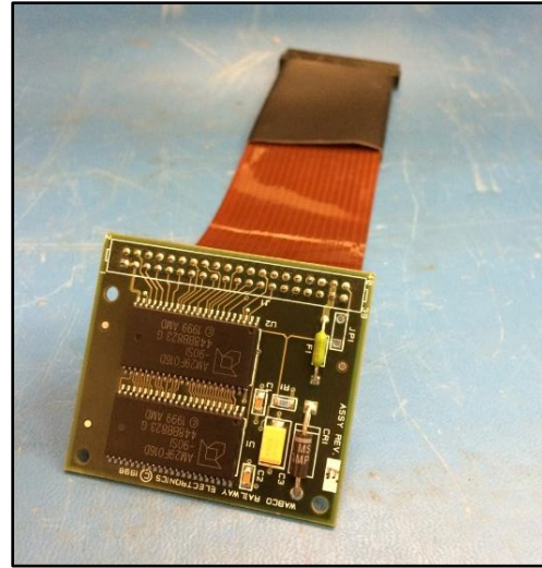
Figure 5. BNSF 3967's memory chips removed and placed on surrogate board
