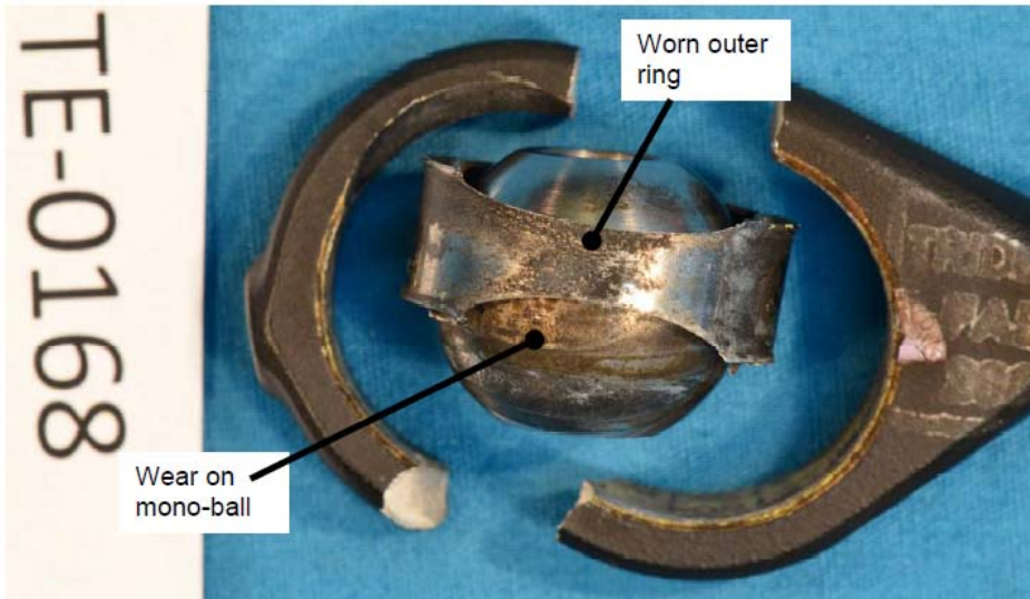
Photo 8. Mechanical contact wear observed on the spherical ball and outer ring of the pitch horn-side spherical bearing of PCL S/N TE-0168. (photo courtesy of Bell Helicopter)
