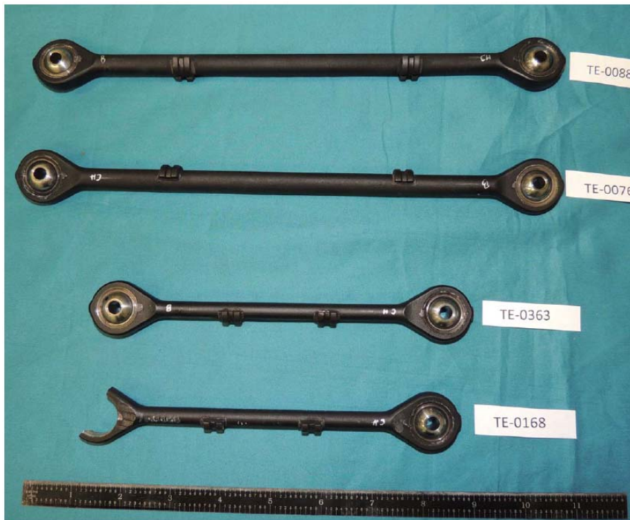
Photo 3. The tail rotor PCLs identified by S/N. (photo courtesy of Bell Helicopter)
