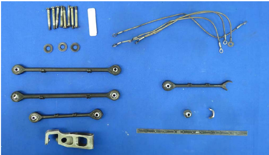
Photo 2. The tail rotor directional control components received at Bell Helicopter facilities. (photo courtesy of Bell Helicopter)
