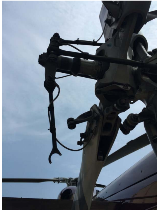
Photo 1. Photo of the fractured tail rotor PCL still installed on N429AR. (photo courtesy of Bell Helicopter)
