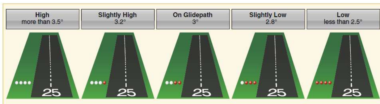
Figure 2: 4-Light Precision Approach Path Indicator (PAPI) 47
