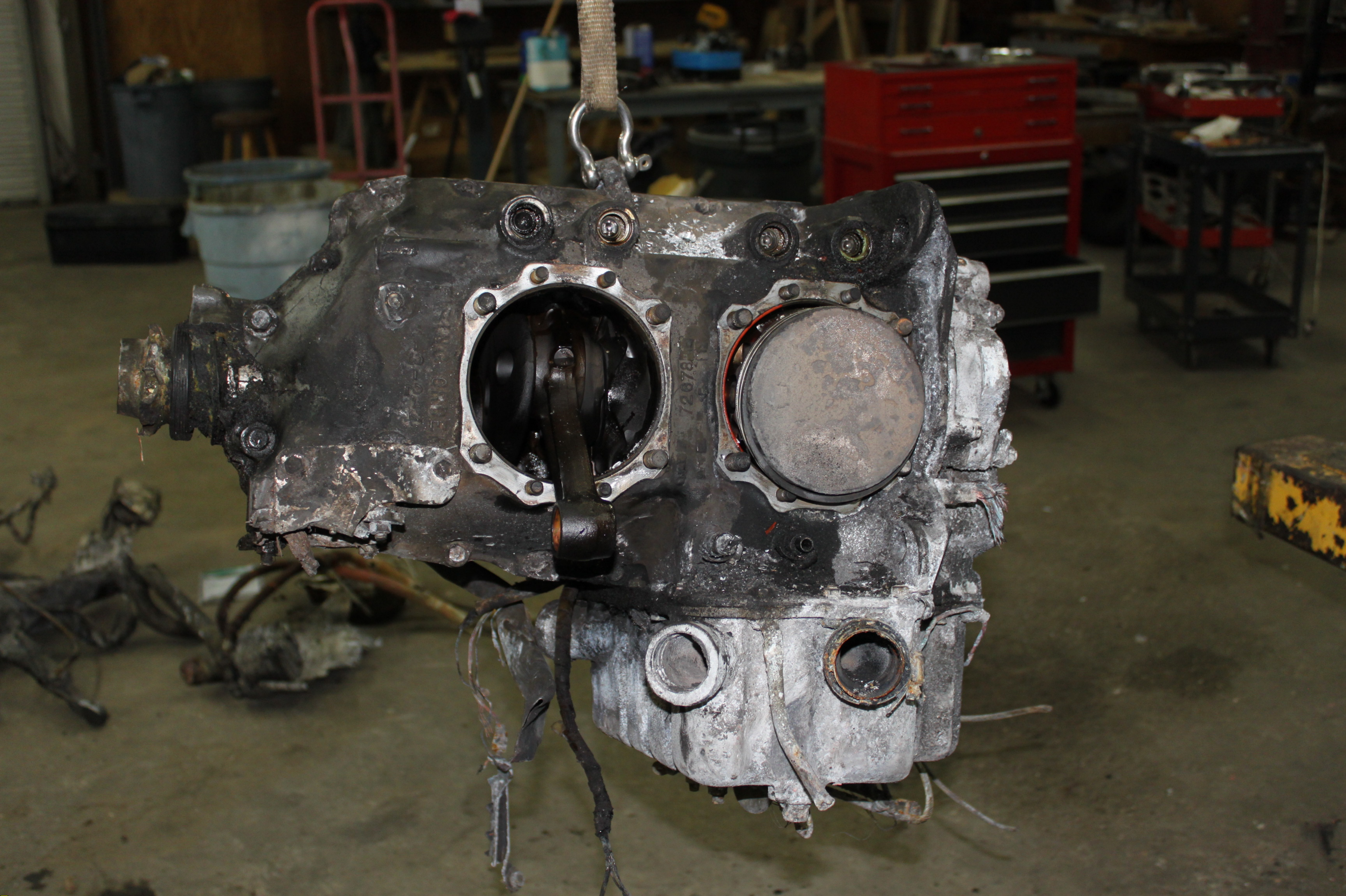
Photo 13: NTSB Digital Photograph, View of the Engine Assembly with the Nos. 2 and 4 Cylinders Removed.
