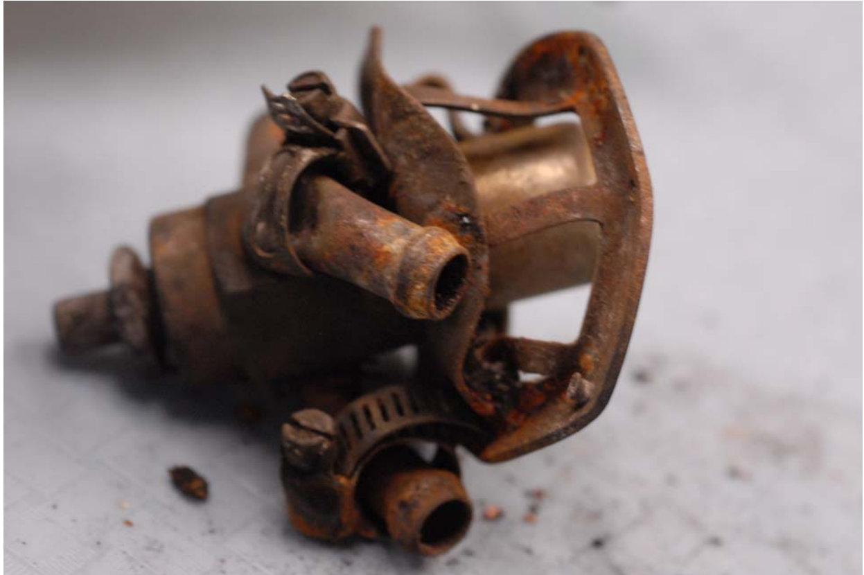
N5714W_10Jun_D019, Vacuum Regulator as received
