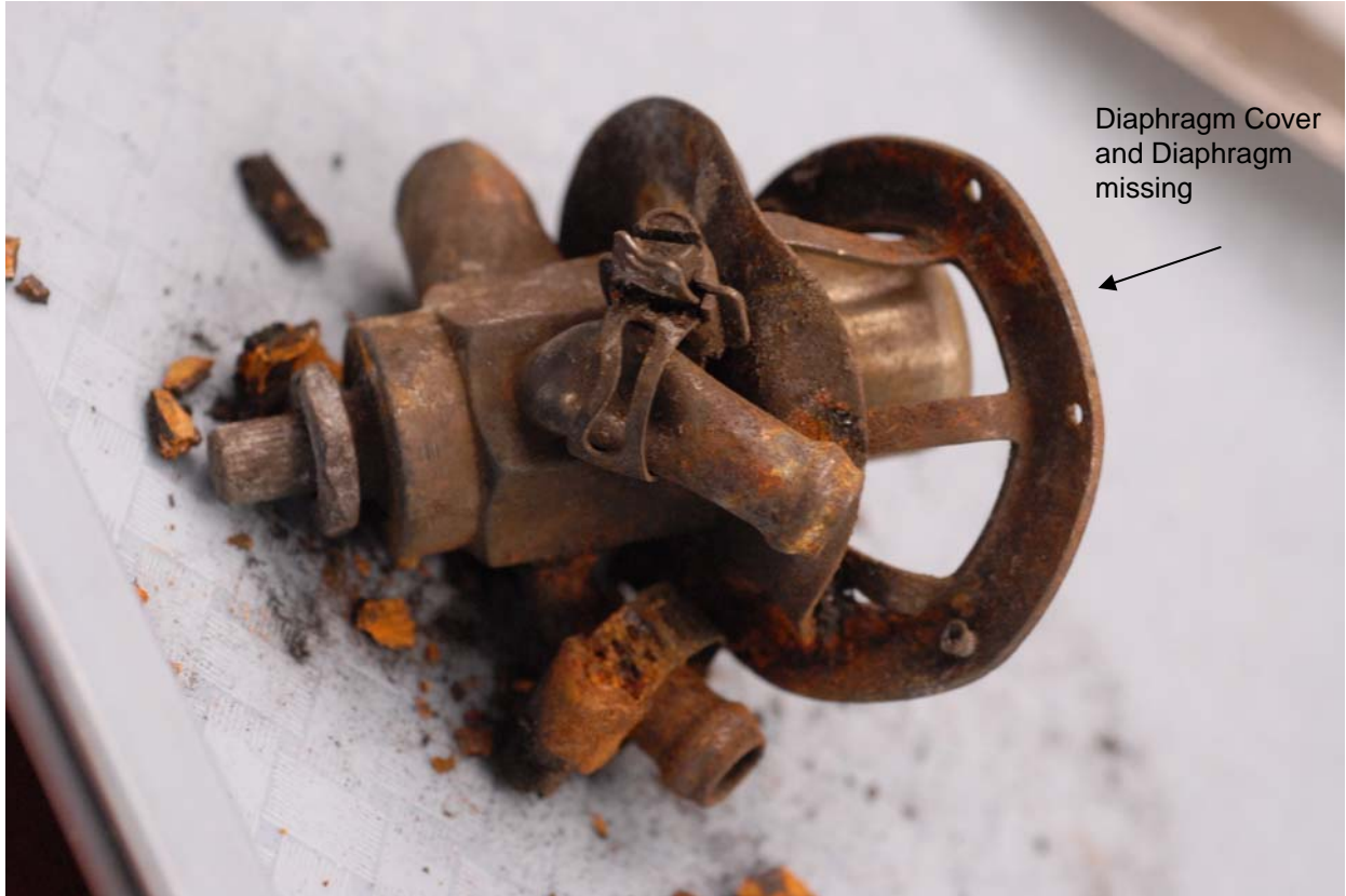
N5714W_10Jun_D009, Diaphragm Cover and Diaphragm missing
