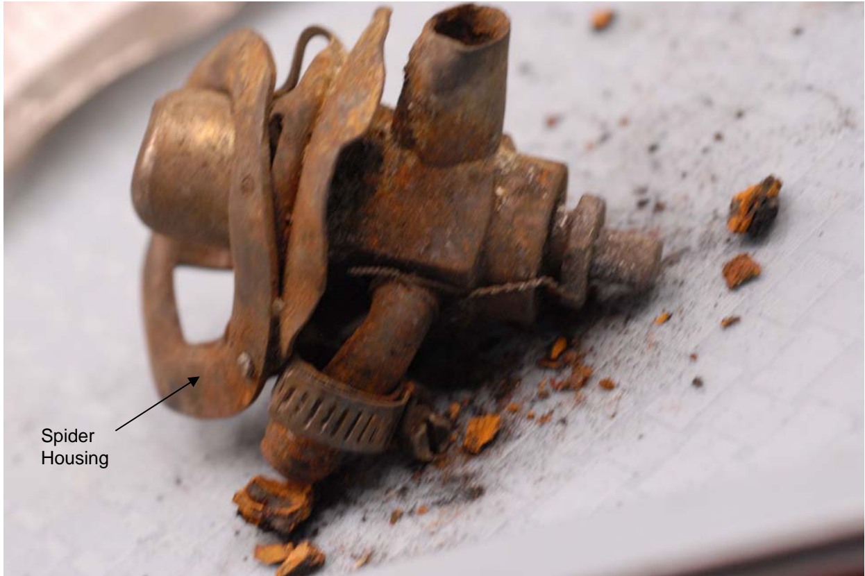
N5714W_10Jun_D010, Spider Housing Crushed
