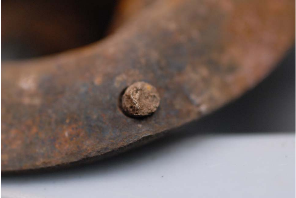
N5714W_10Jun_D023, Rivet for attaching Diaphragm and Diaphragm Cover
