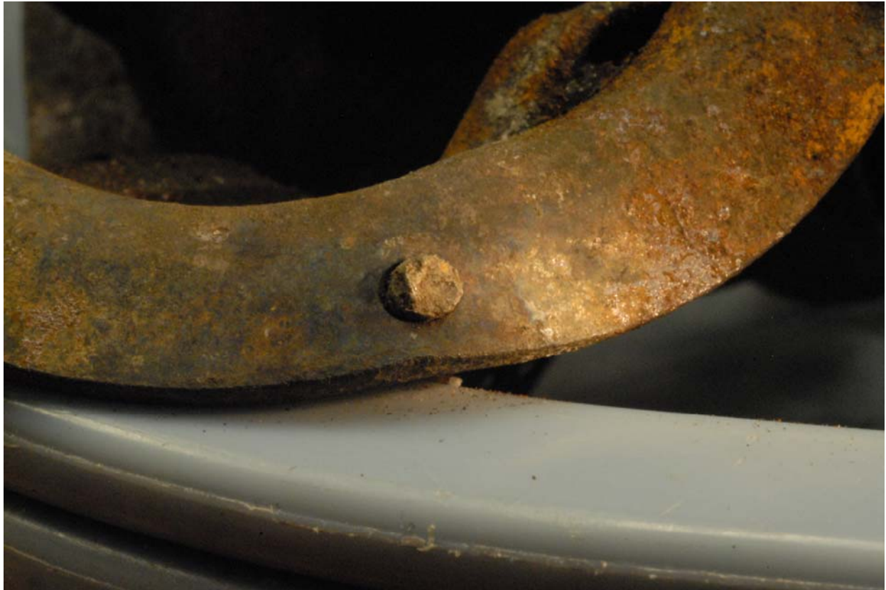
N5714W_10Jun_D025, Rivet for attaching Diaphragm and Diaphragm Cover
