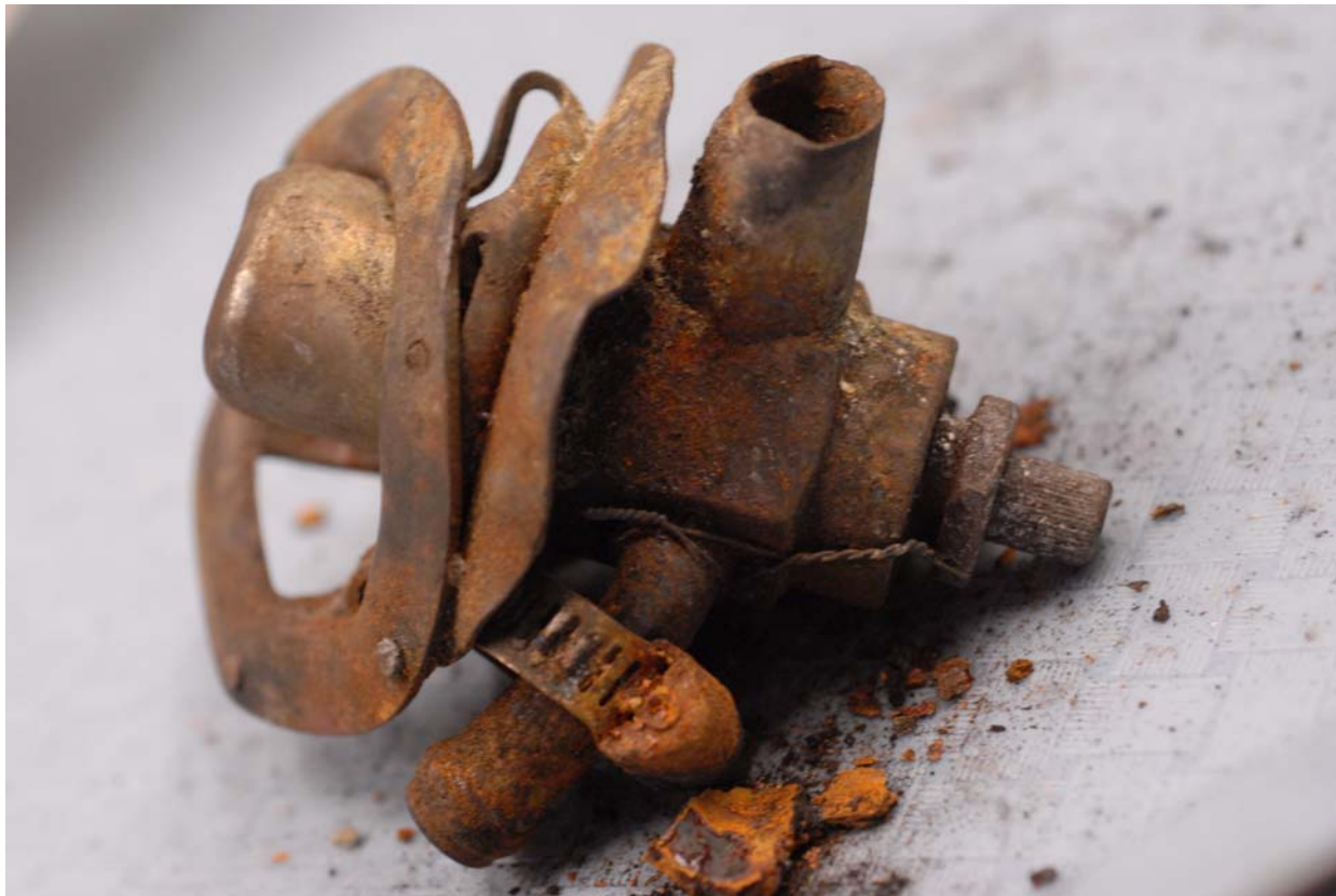
N5714W_10Jun_D017, Vacuum Regulator as received
