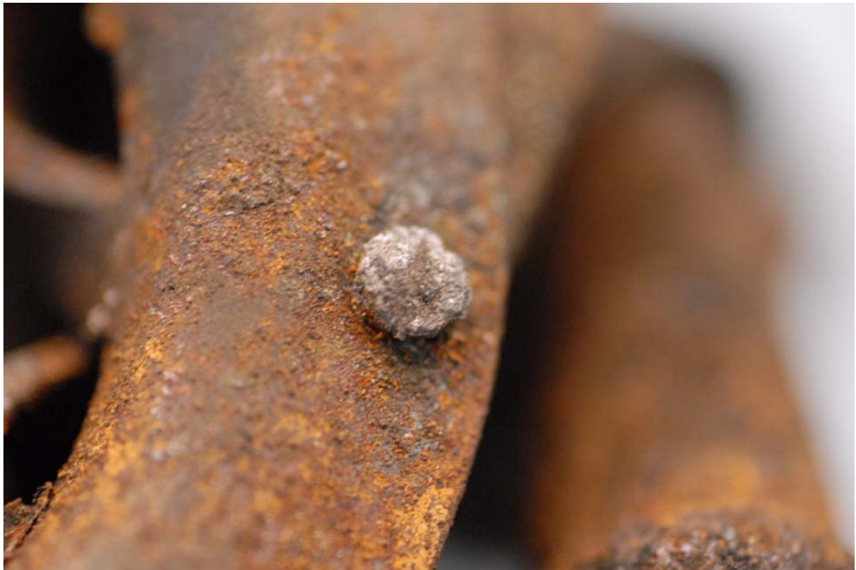
N5714W_10Jun_D022, Rivet for attaching Diaphragm and Diaphragm Cover
