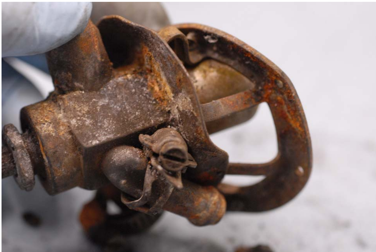
N5714W_10Jun_D018, Vacuum Regulator as received
