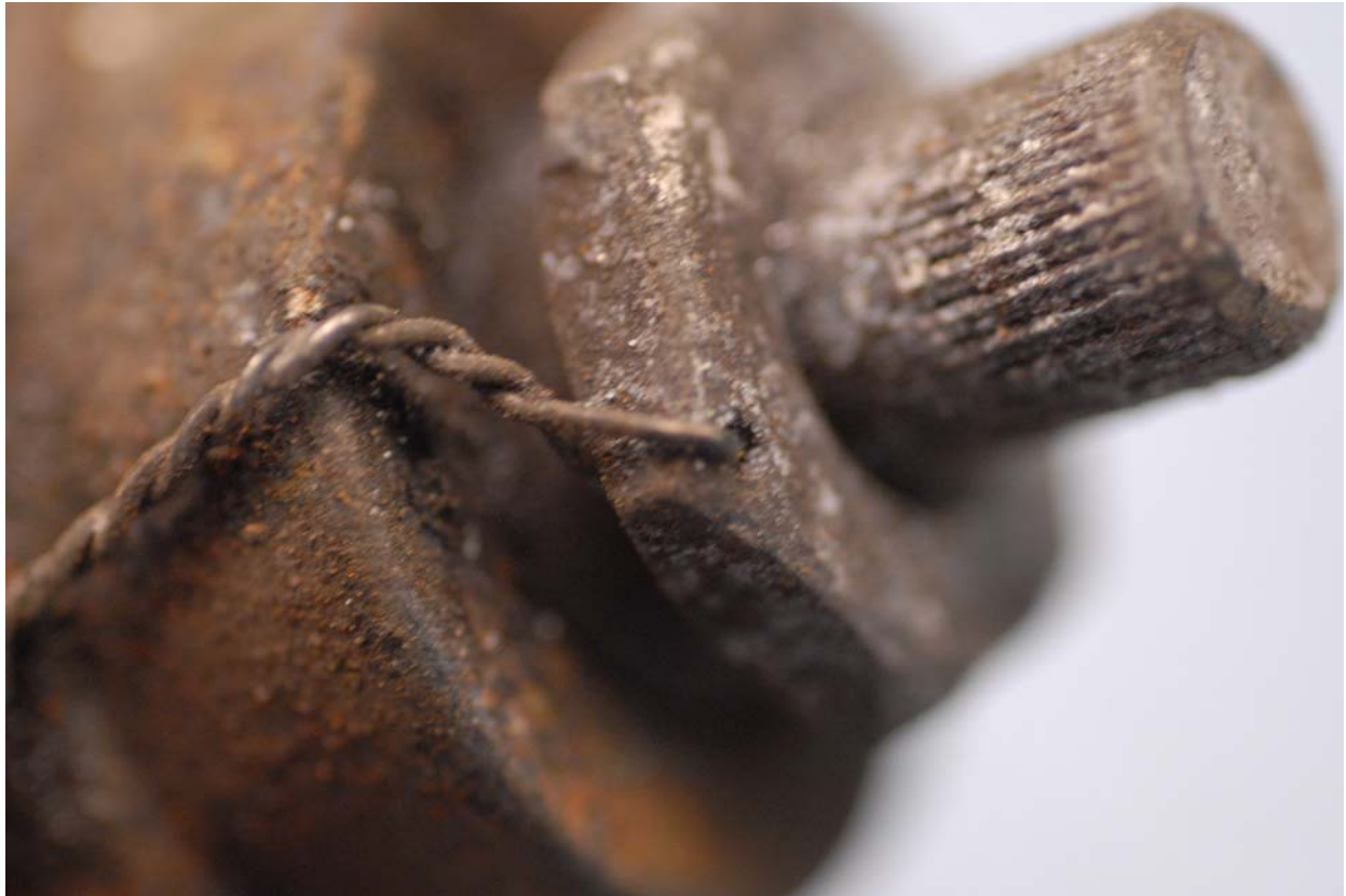
N5714W_10Jun_D012, Lock Wire in place
