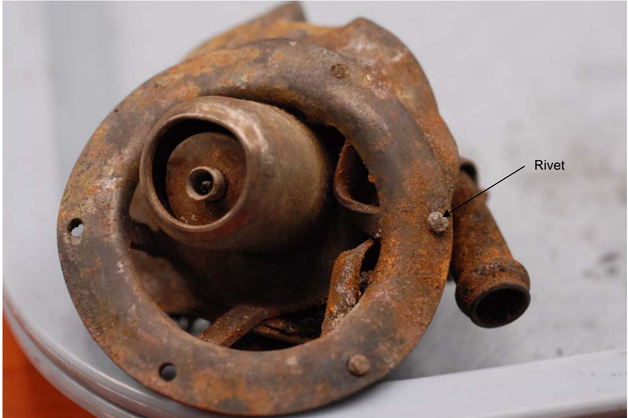
N5714W_10Jun_D021, Rivets for attaching Diaphragm and Diaphragm Cover
