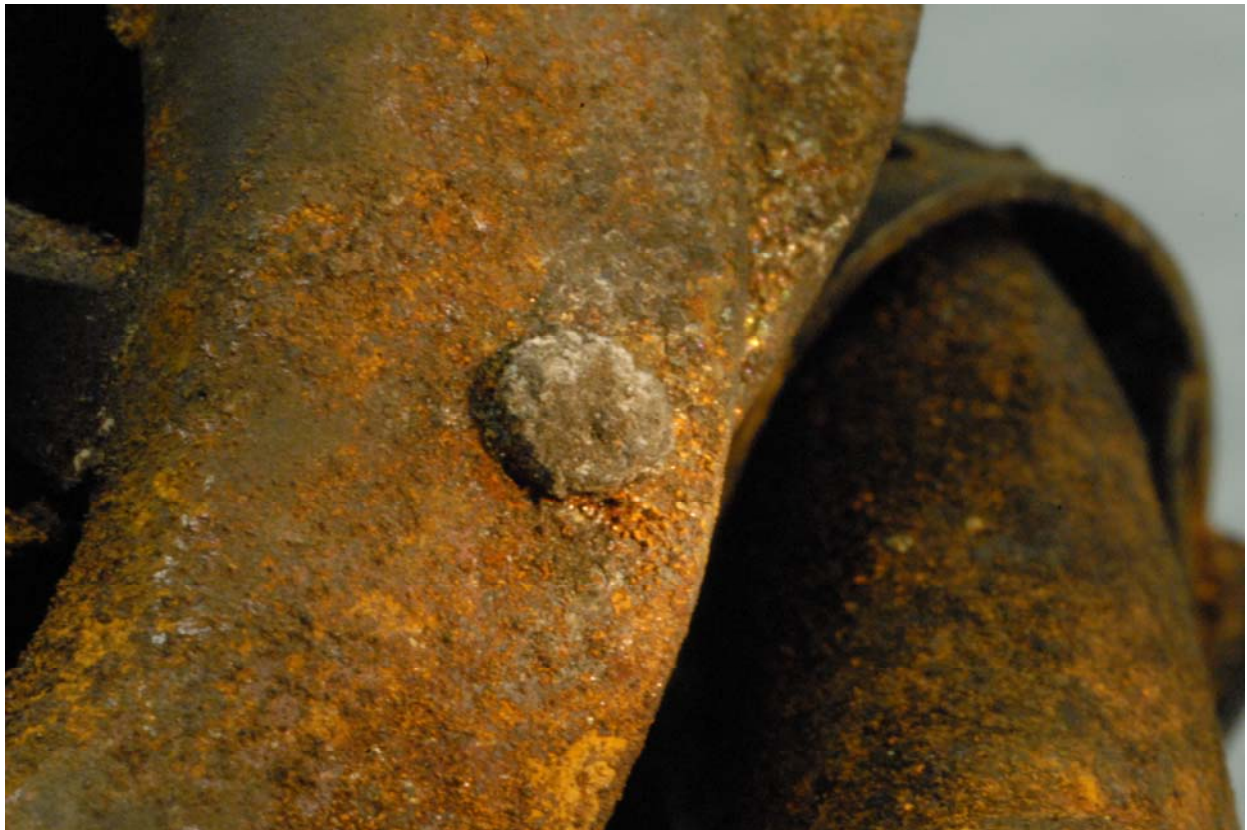
N5714W_10Jun_D024, Rivet for attaching Diaphragm and Diaphragm Cover
