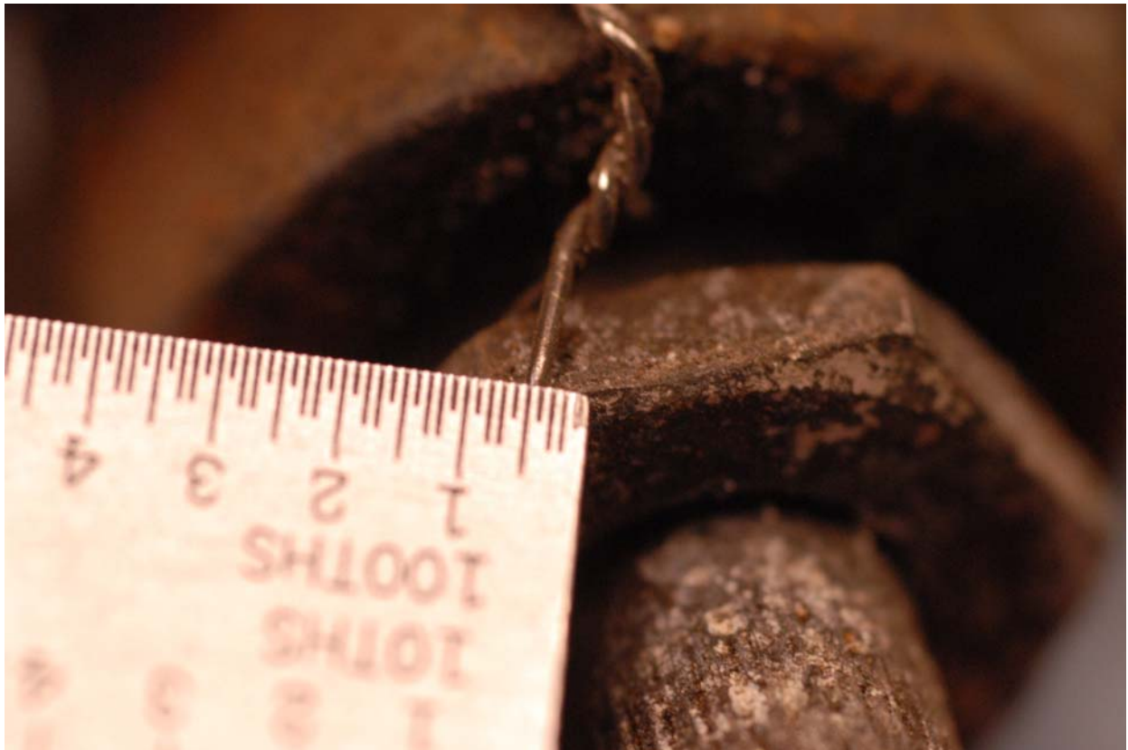
N5714W_10Jun_D020, Lock wire Diameter
