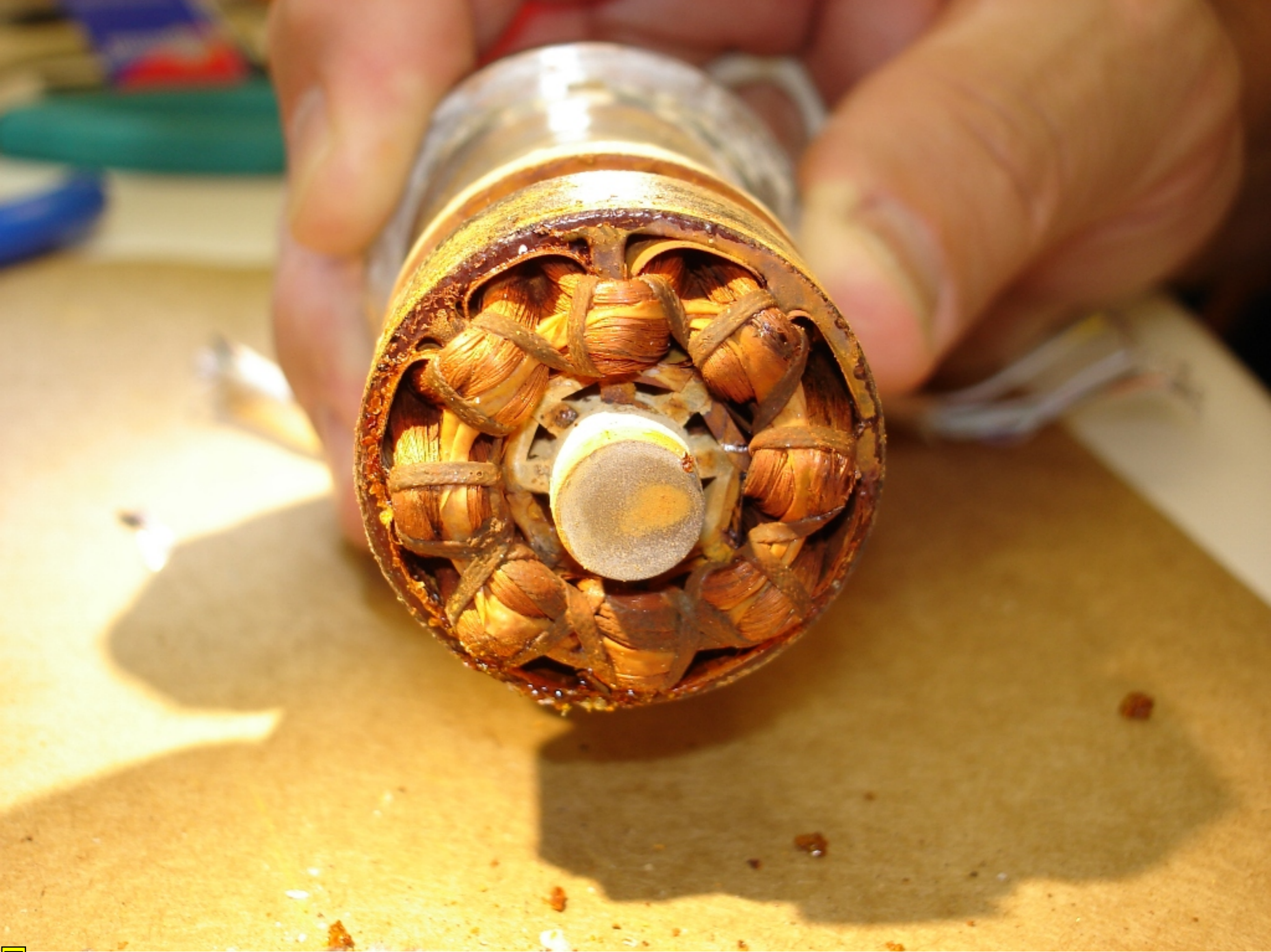
Photo 14. View of the electrical motor of the stepper motor.
