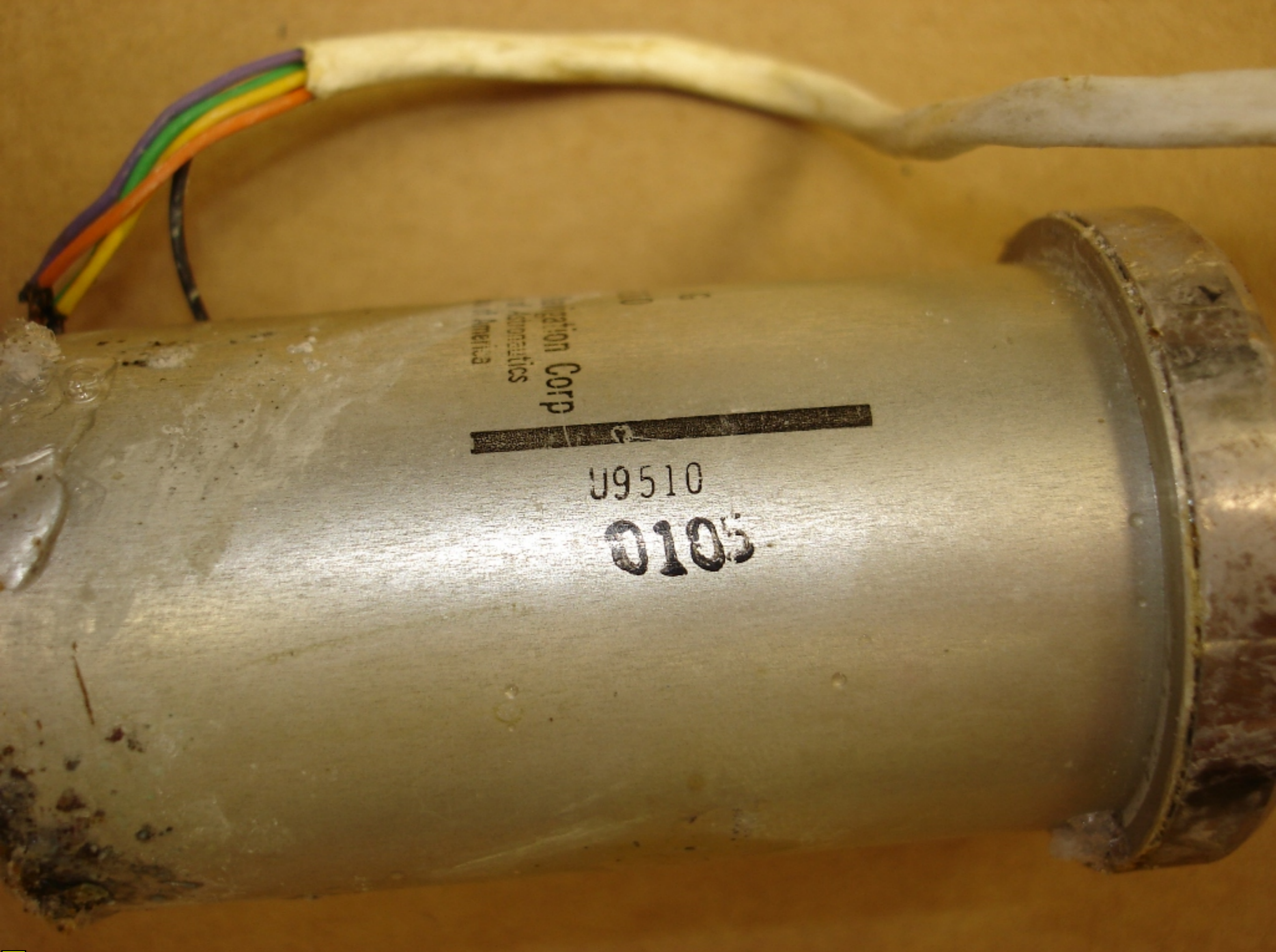
Photo 10. Stepper motor of the right engine fuel control.
