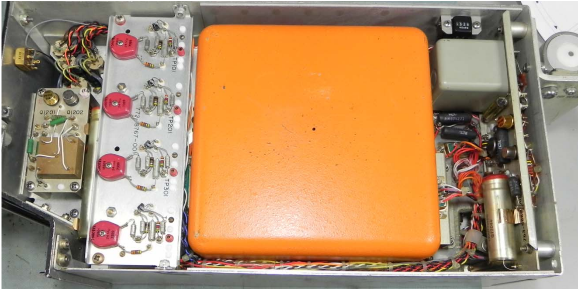
Figure 1. Interior of unit showing crash protected tape housing.
