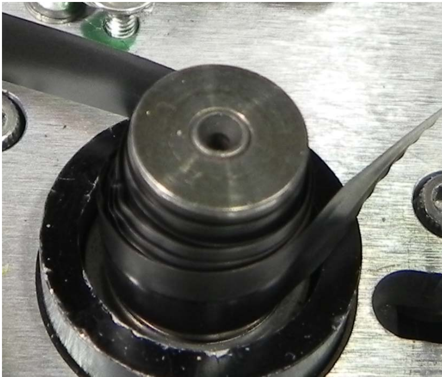
Figure 5. Final spindle with tape tensioner removed.
